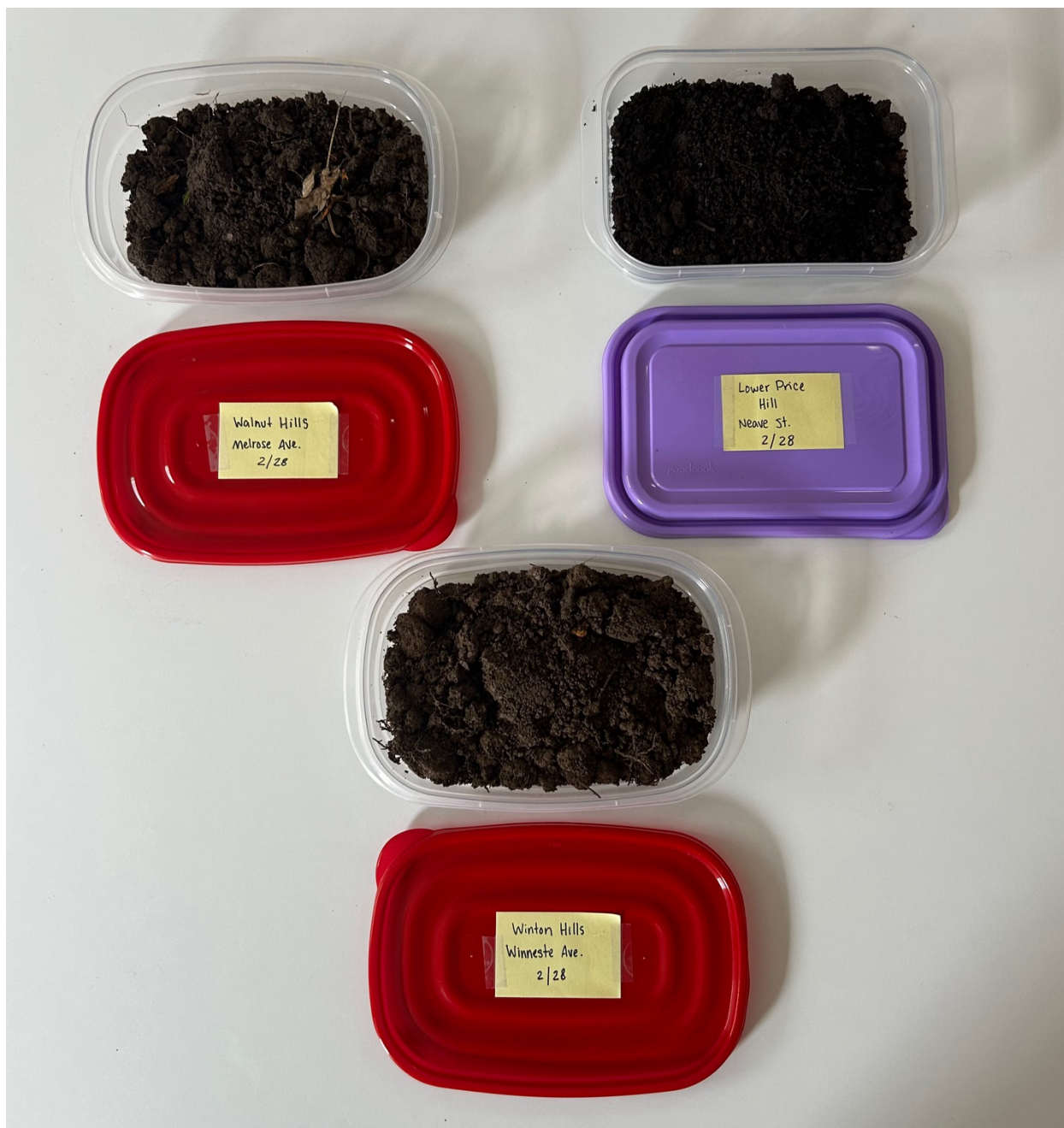
Figure 37: Soil Samples Placed in Containers to Air Dry for 72 Hours
