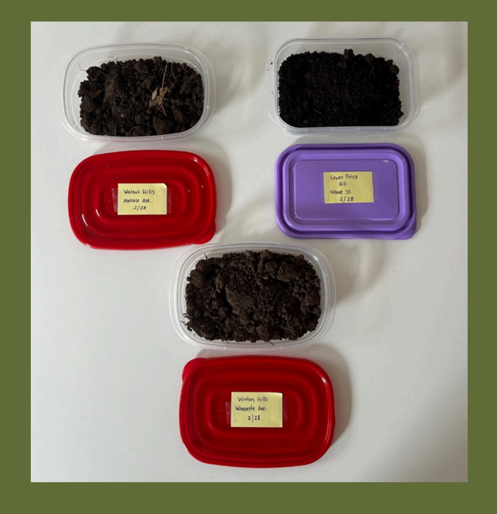
Figure 20: Soil samples placed in containers to air dry for 72 hours
