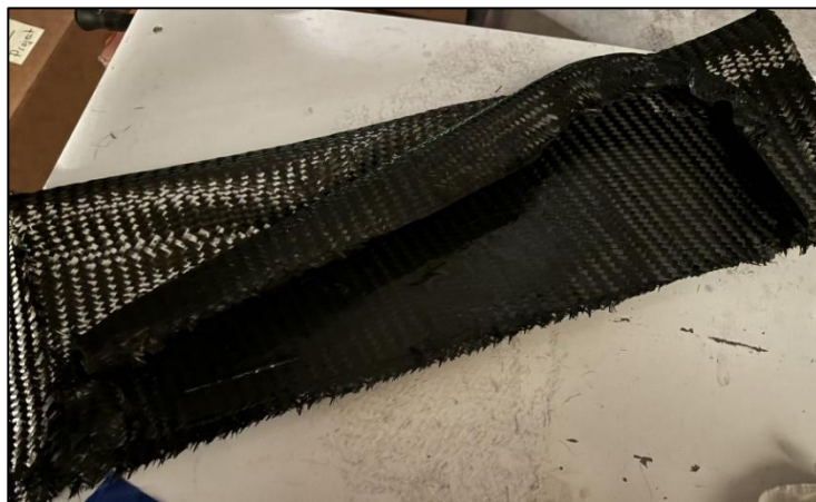
Figure 20: Carbon Fiber Chain Guard
