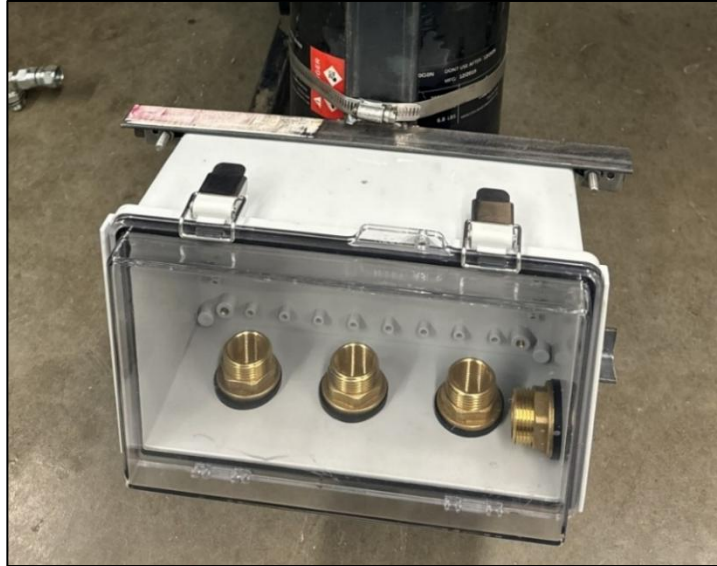
Figure 19: Clear conduit box used as our hydraulic fluid reservoir
