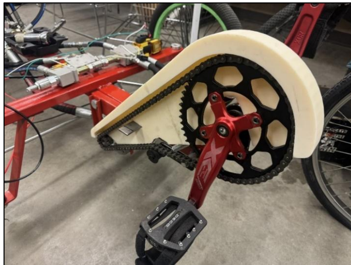
Figure 17: 3D Printed ABS Chain guard
