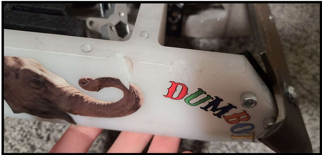
Figure 33: Additional damage from impacts
