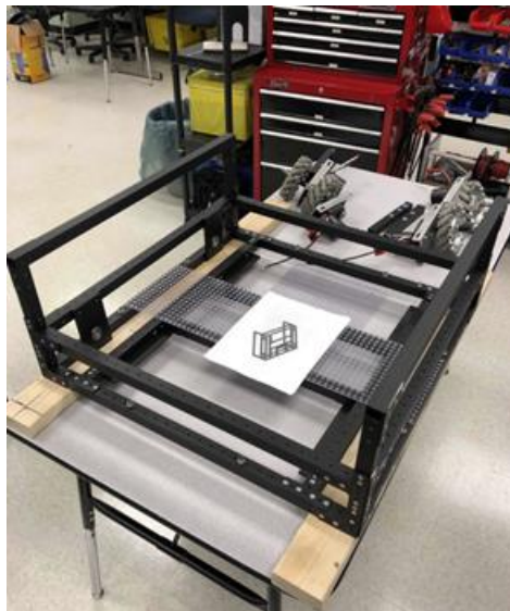
Figure 1: Kyber Robot Aluminum Riveted Frame
