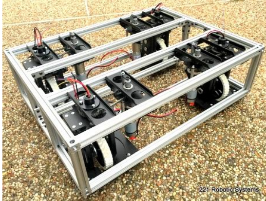
Figure 3: Swerve/Crab Platform Aluminum Extrusion Frame
