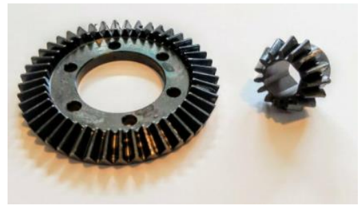
Figure 23: AISI 1045 Alloy Steel Bevel Gears
