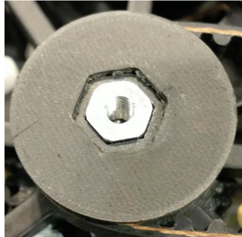
Figure 73: Metal Insert Installed into Drive Pulley
