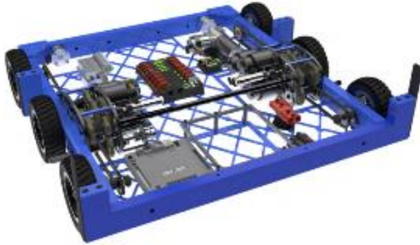
Figure 2: Dreadnought Robot Aluminum Welded Frame
