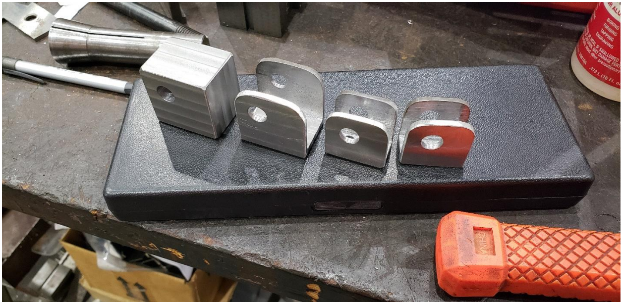
Figure 7 – Machining of Bushing and Damper Brackets
