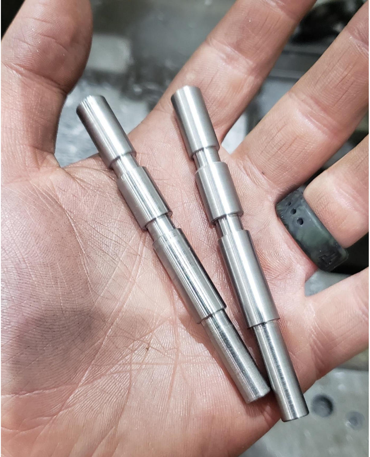
Figure 10 – Completed Turning Operation on Damper-Band Shanks
