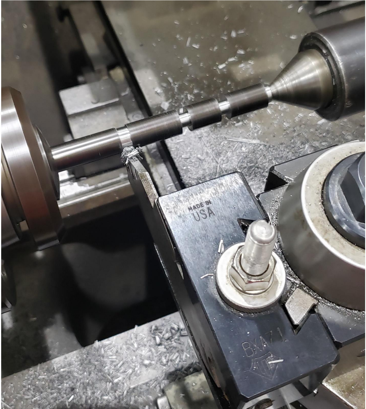
Figure 9 – Turning Damper-Band Shanks on Clausing Lathe
