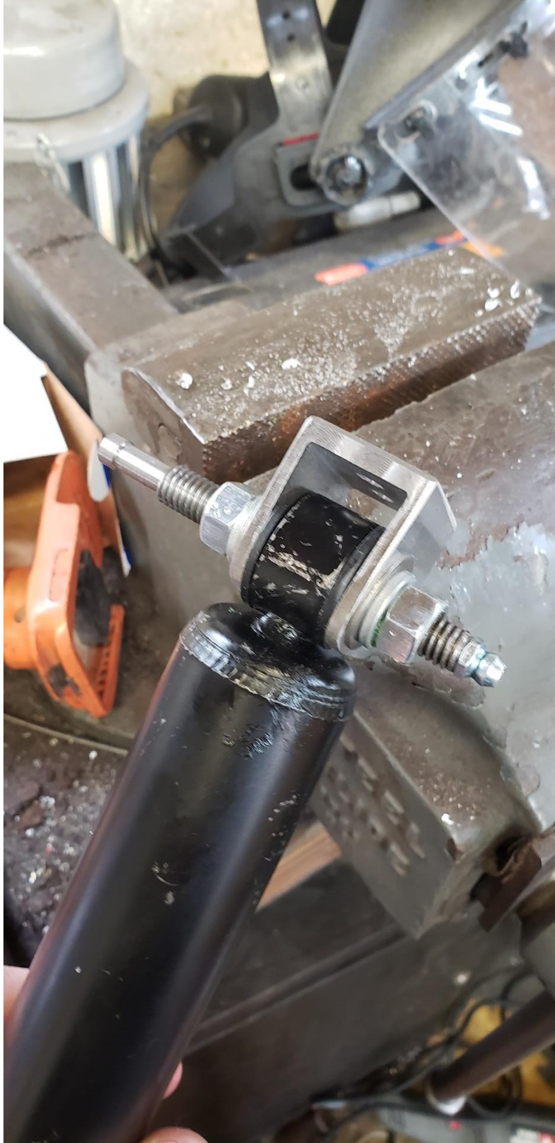
Figure 11 – Test Fit of Damper, Bracket, and Shank
