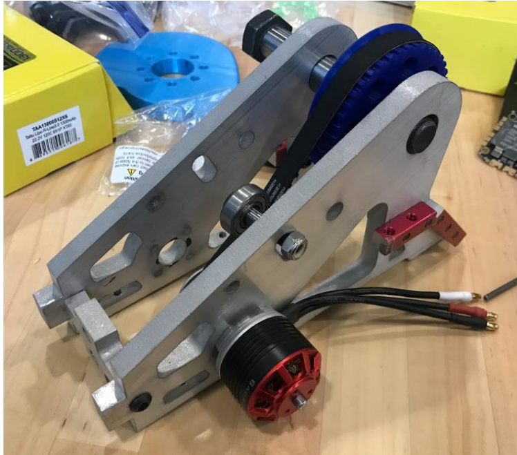
Figure 4.62: Weapon Motor Fastened to Upright
