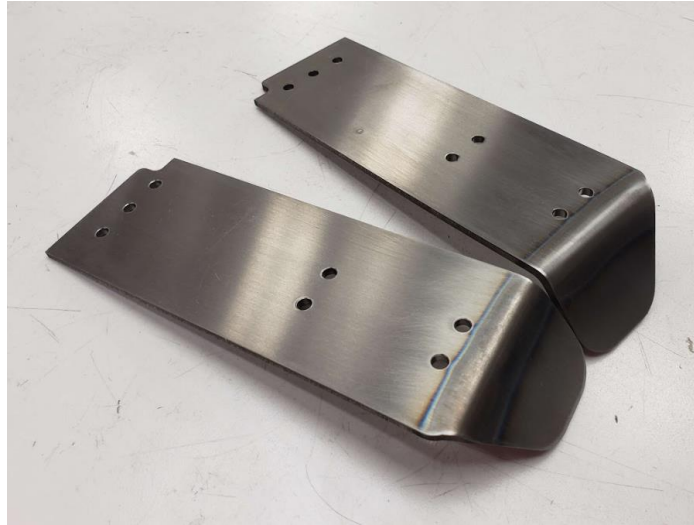
Figure 4.39: 50 Degree Torch Bent Titanium Wedges
