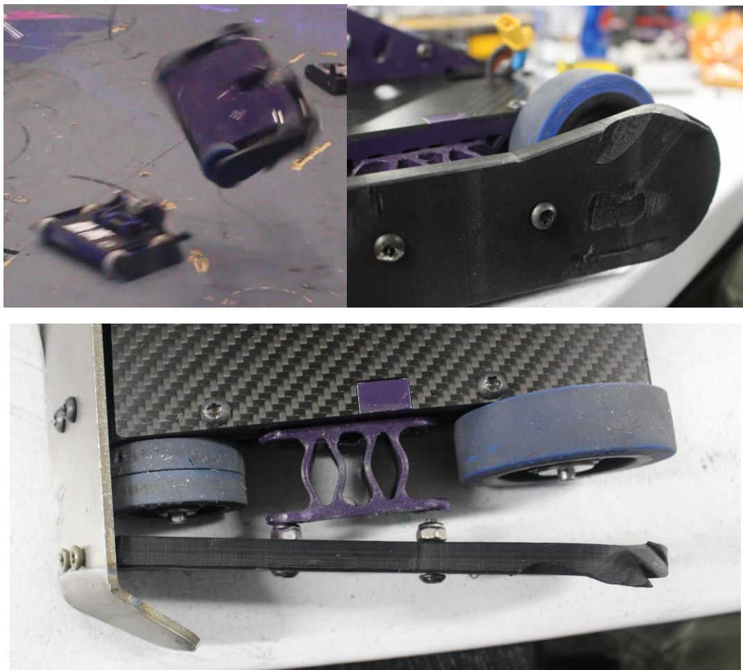
Figure 4.80: Saiko!'s Hit on Voodoos UHMW Side Armor and Resulting Damage
