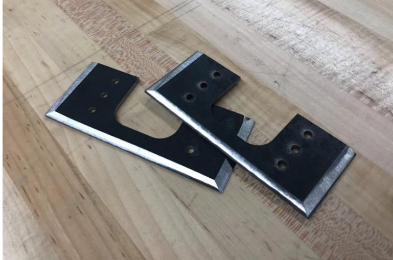
Figure 4.41: Sharpened AR500 Horizontal Blade Deflectors
