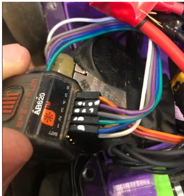
Figure 4.52: Labeled Signal Wires Plugged into AR620 Receiver
