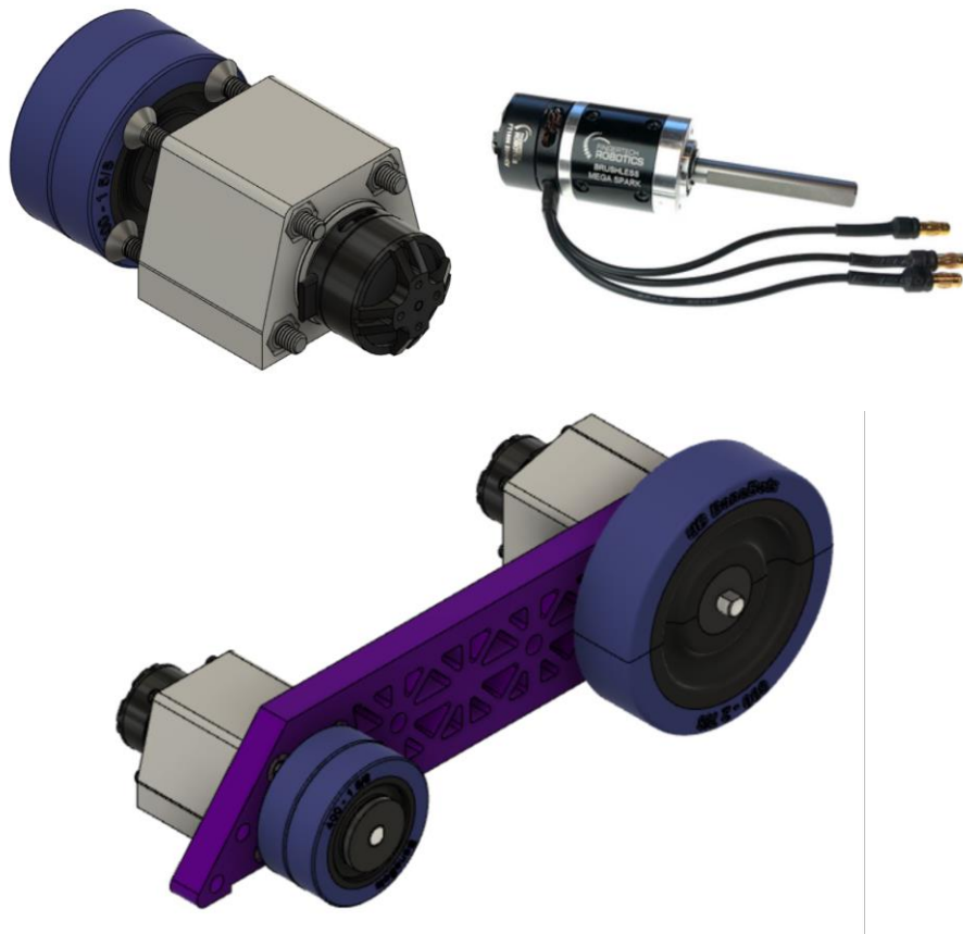
Figure 4.2: Drivetrain Sub-Assembly and Drive Motor
