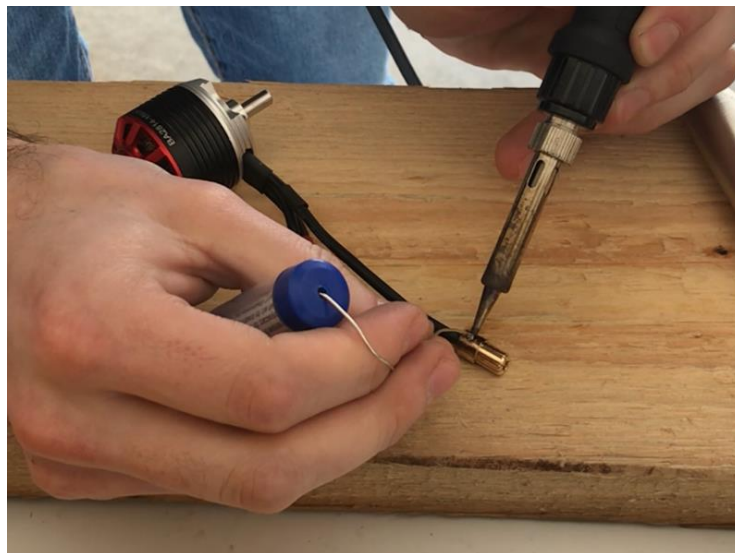
Figure 4.50: Soldering 6.5mm Bullet Connector to Weapon Motor
