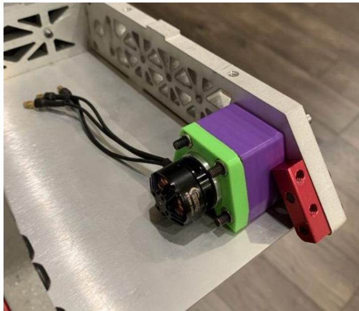
Figure 4.63: Drive Module Fastened to Side Plate
