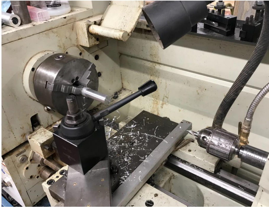
Figure 4.47: Turning Down and Boring Weapon Spacers on Lathe
