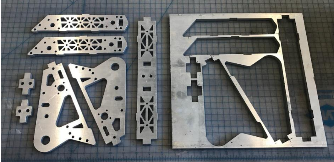
Figure 4.28: Post waterjet cutting of the frame with the leftover stock material
