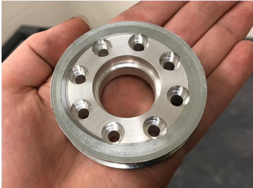
Figure 4.45: Boring Bearing Hole and Counter bores into Pulley
