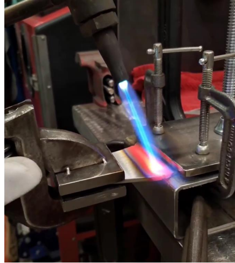
Figure 4.23: Complete Wedge Model and Torch Bending Titanium Wedge
