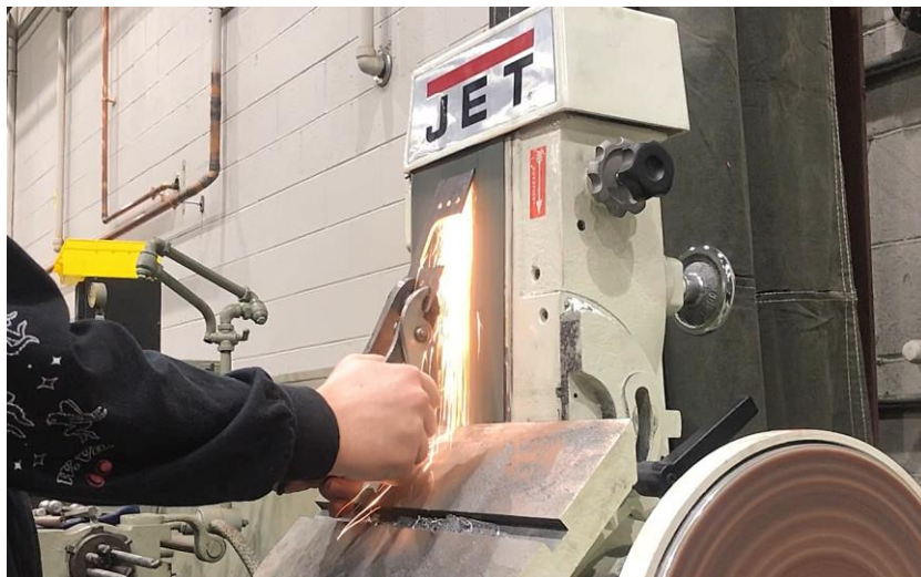
Figure 4.40: Grinding AR500 Horizontal Blade Deflectors
