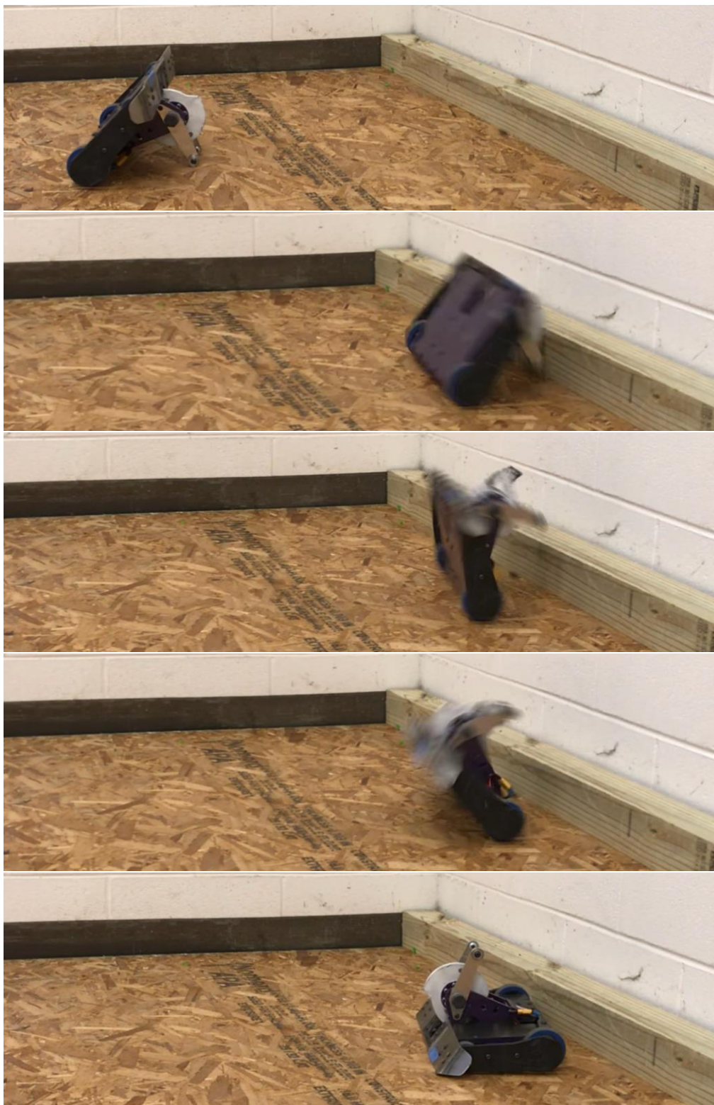
Figure 4.74: Self Inverting Test
