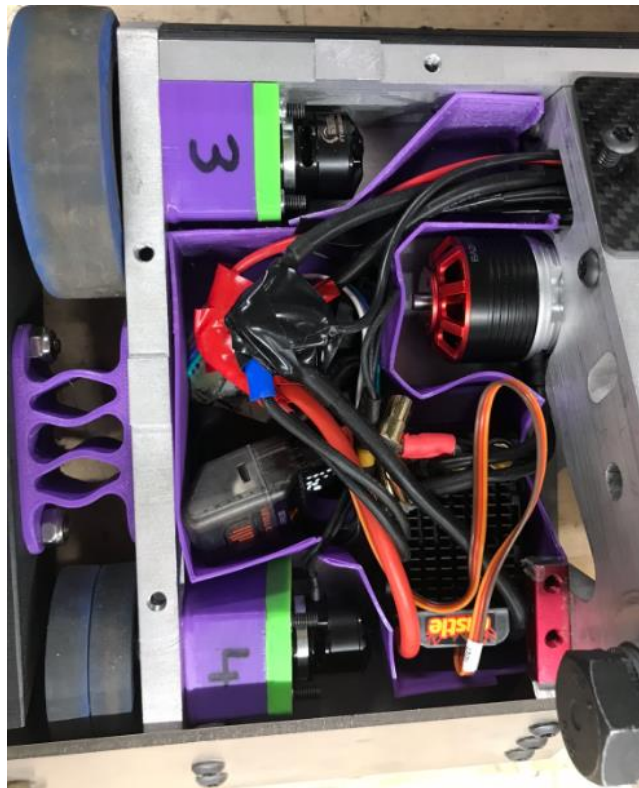
Figure 4.54: Complete Wiring Harness Installed in the Robot
