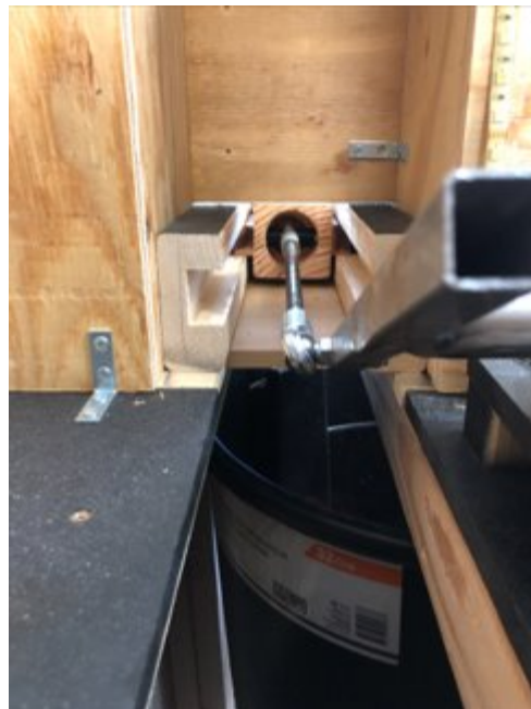
Figure 19 - Final Crushing Chamber Design
