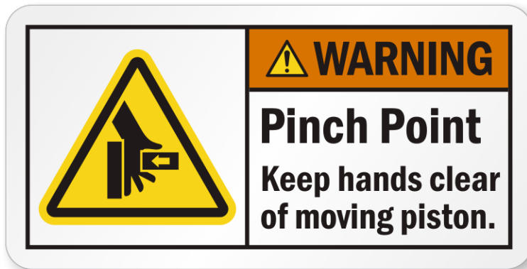
Figure 21 - Pinch Point Warning
