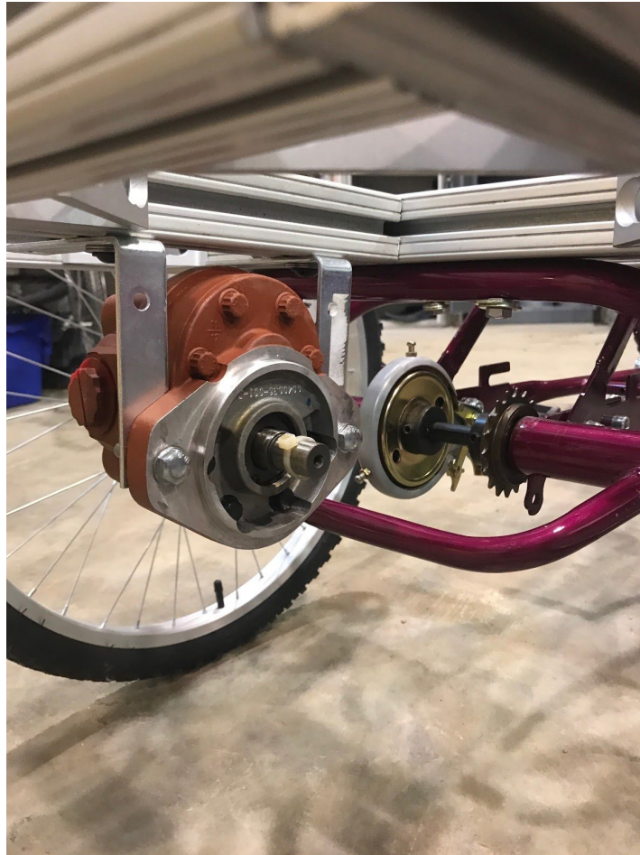
Figure 11: Placement of the motor on the underside of the 80/20 frame.
