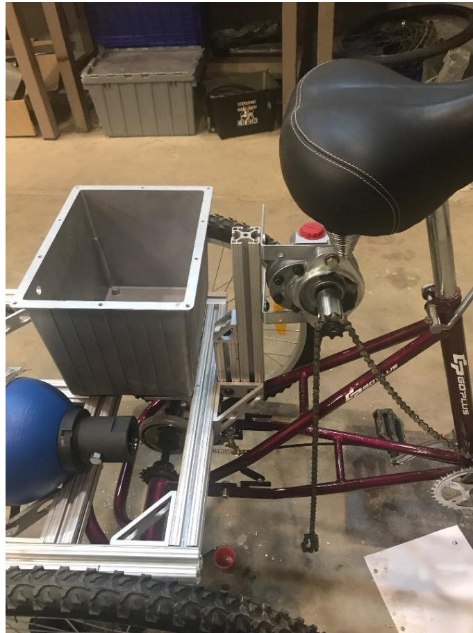
Figure 10: Placement of the pump and the reservoir.
