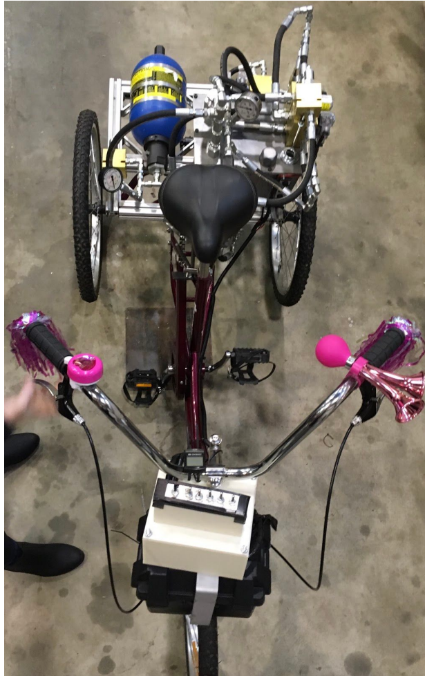
Figure 12: Placement of the accumulator, battery, PLC, switches, and hoses.
