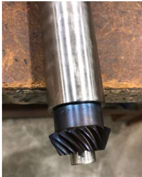
Figure 63 – Gear 2 Heat Shrink Fitting
