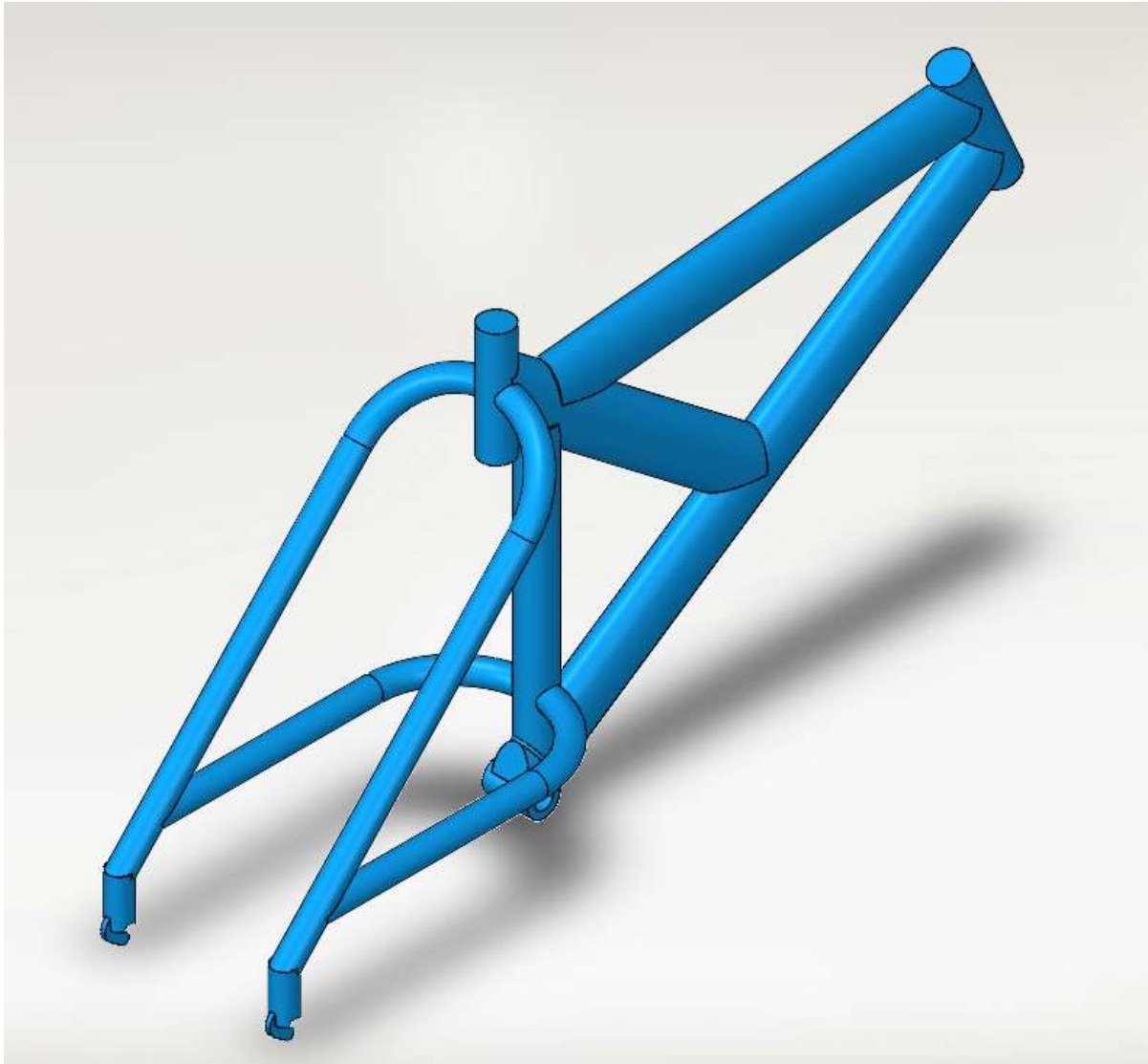
Figure 3 – Bent Pipe Frame Design
