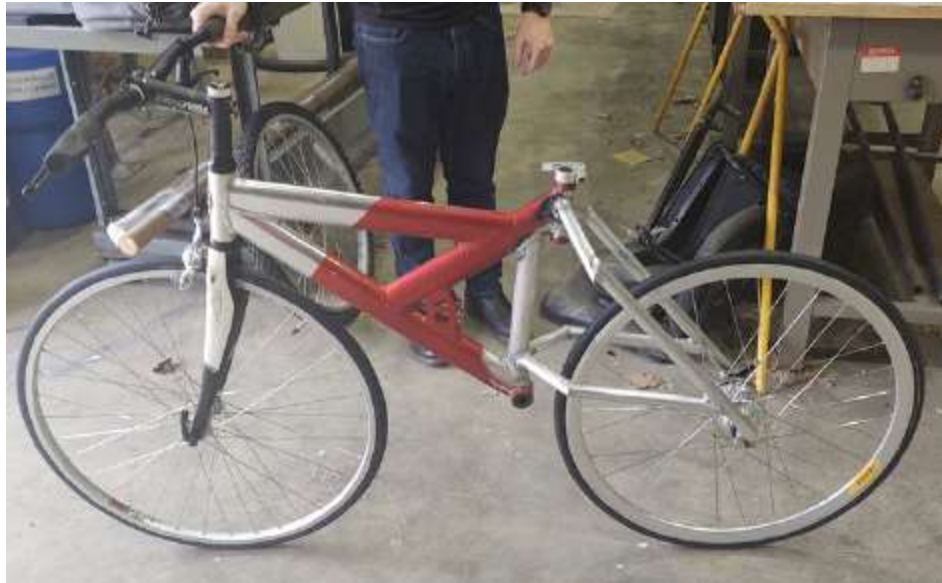
Figure 53 – Welded Bicycle Frame
