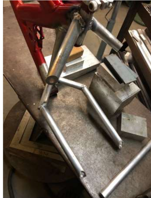
Figure 49 – Lower Rear Fork Welding (Left)
