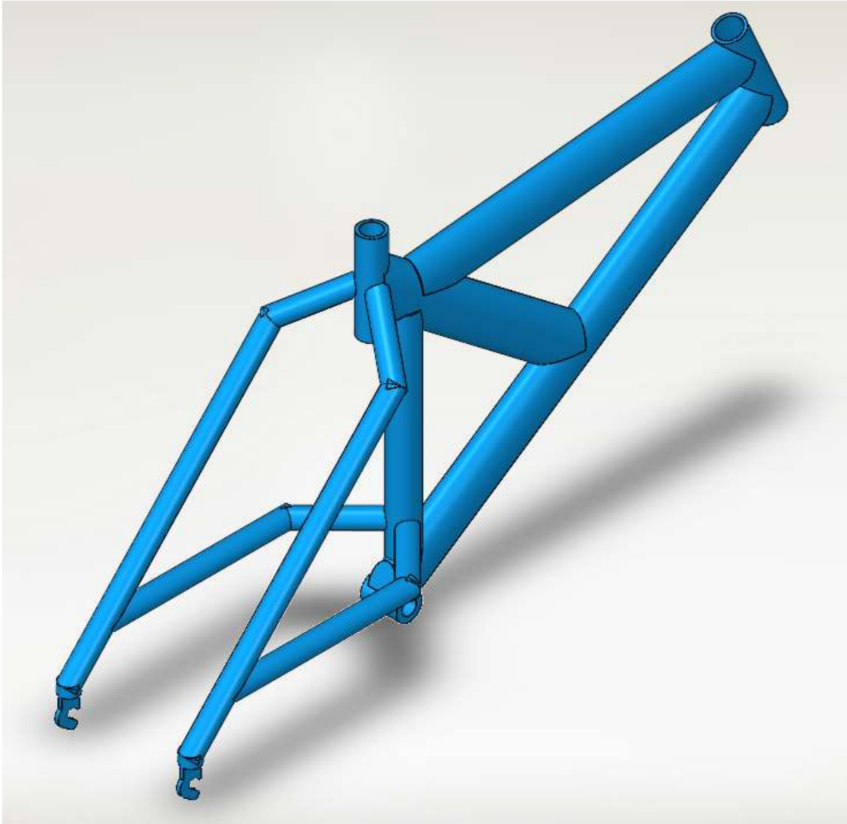
Figure 4 – Cut Pipe Frame Design
