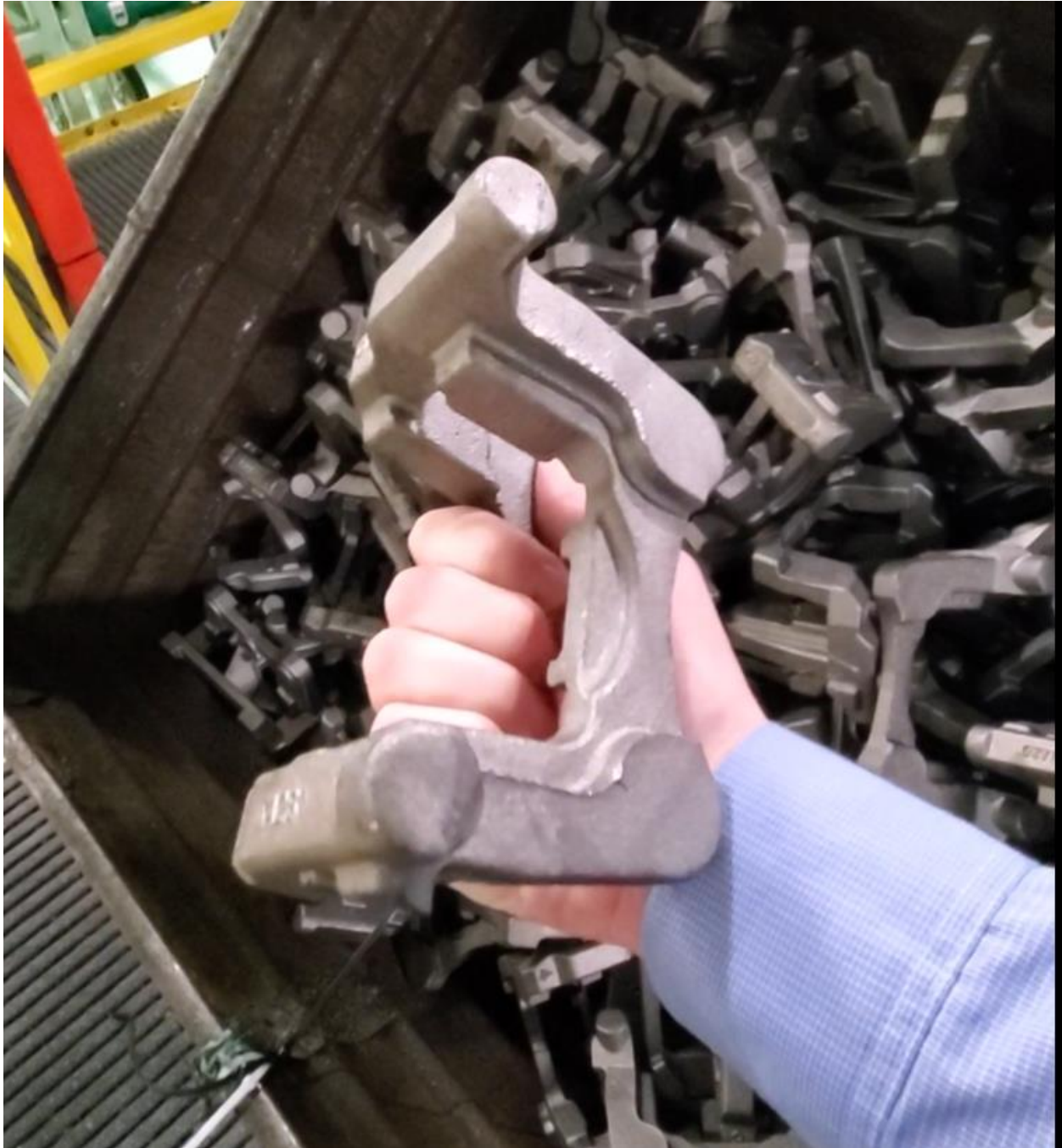
Figure 6 Raw Casting of a Bracket Part
