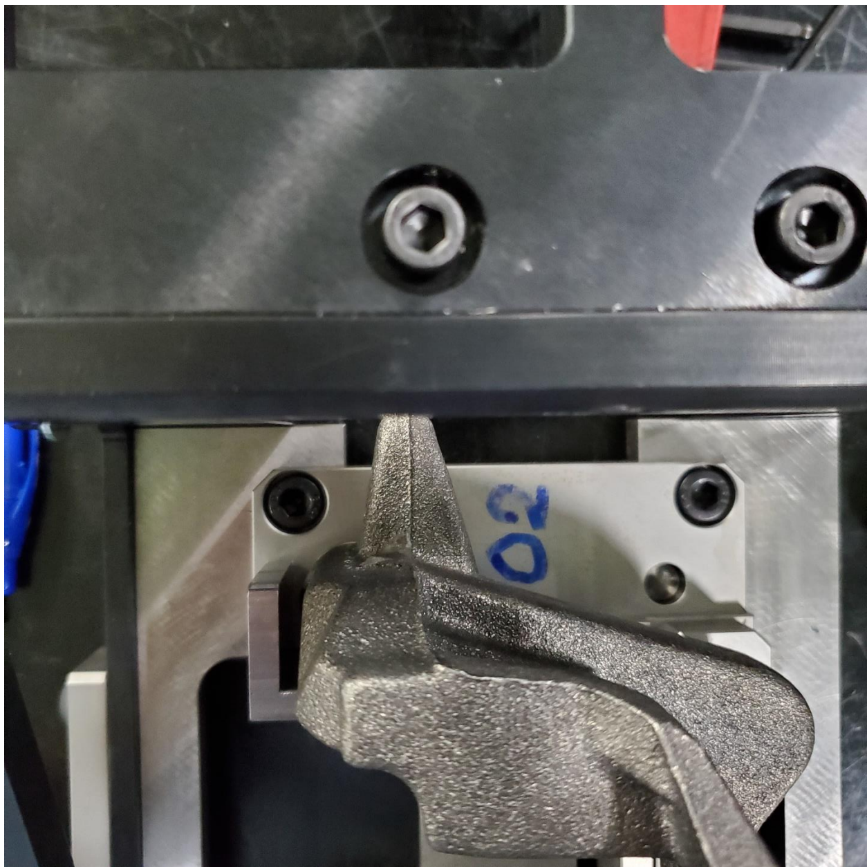
Figure 39 Side Plate Pre Cut
