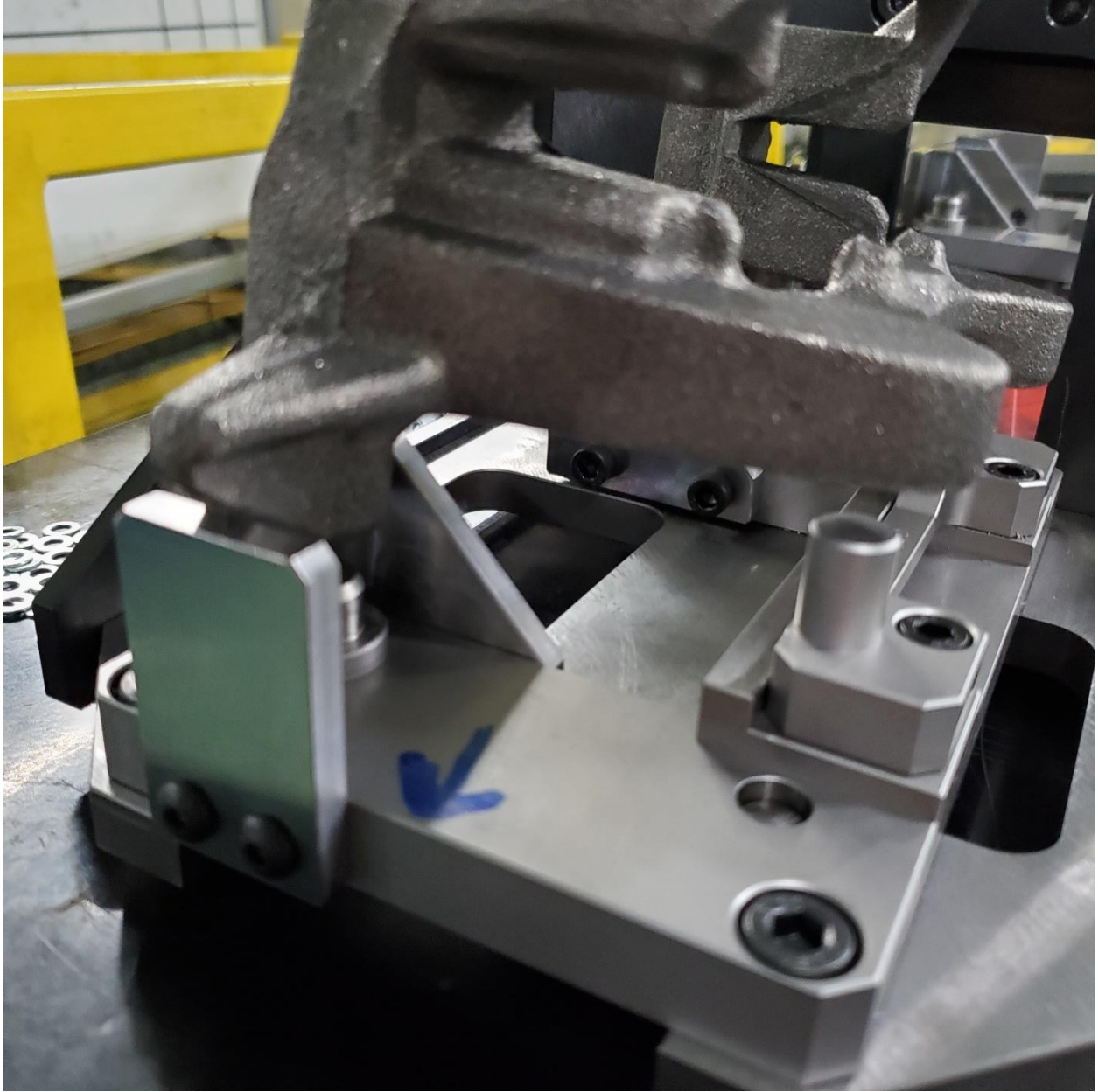
Figure 36 Improperly Placed Corolla Part
