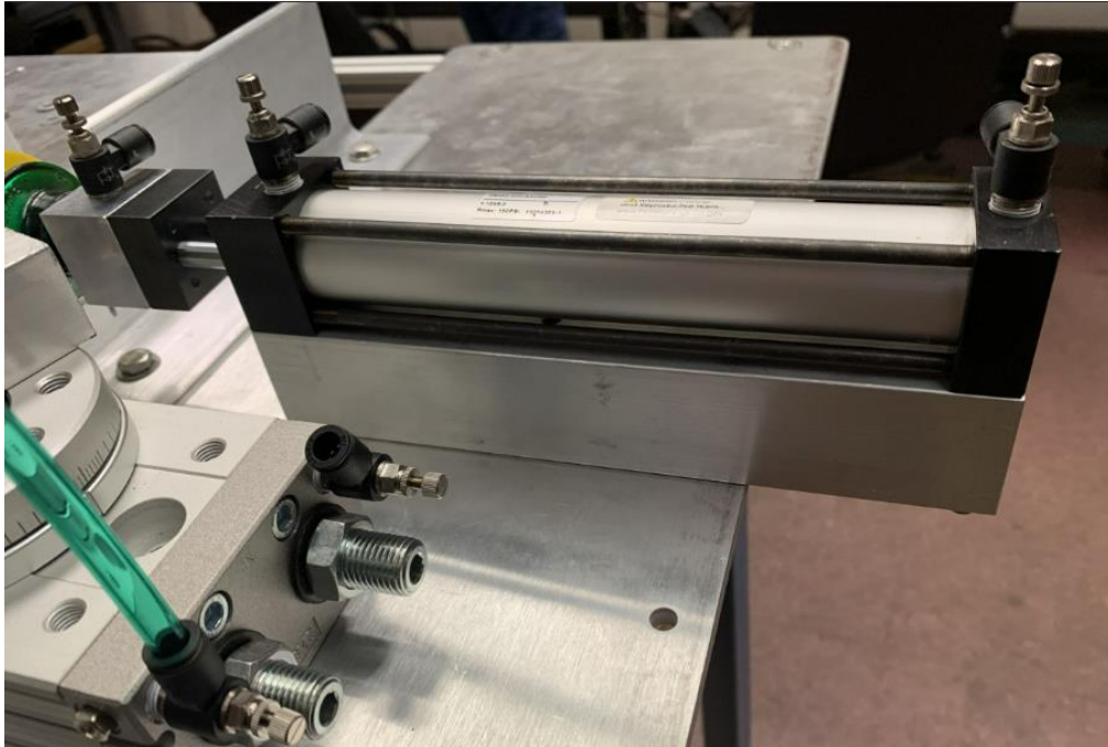
Figure 19: Air cylinder with custom mount allowing it to be raised above the baseplate surface
