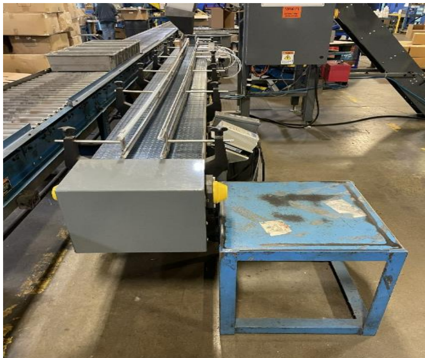
Figure 1: Conveyor belt leading to Vertical Bagger machine
