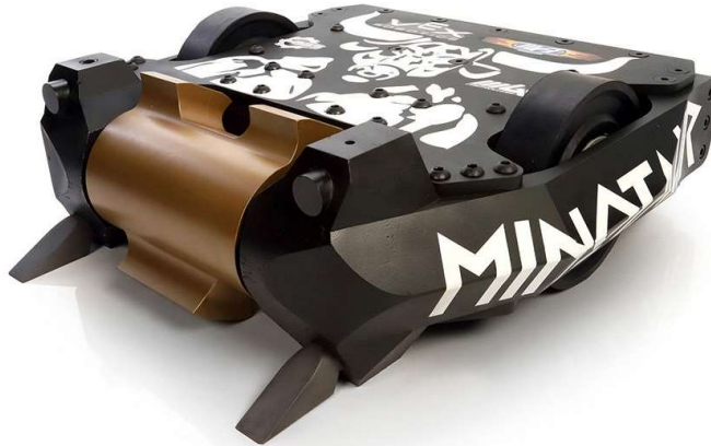
Figure 2. Minotaur, a bot whose powerful drum spinner has earned it 15 wins in only 3 years of combat. (8)
