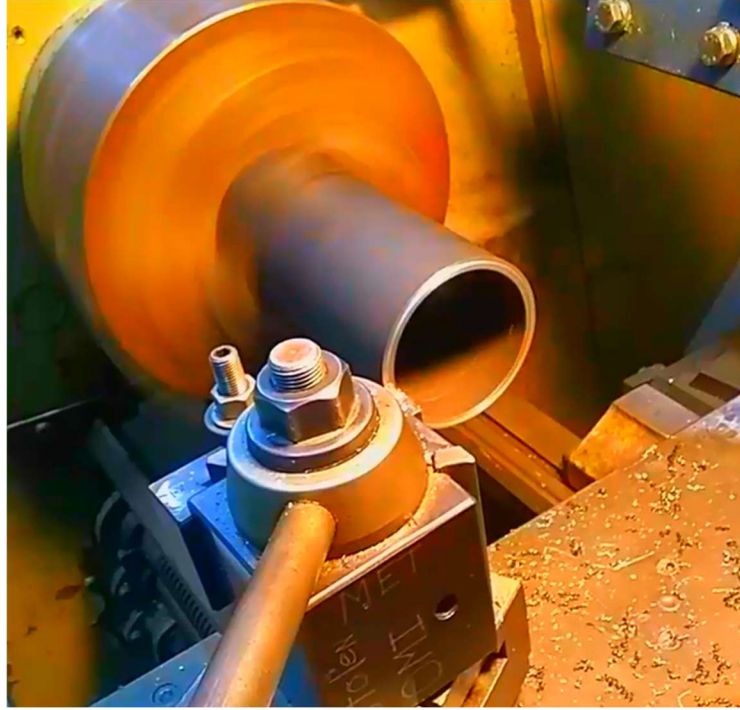
Figure 38. Face cuts on the lathe
