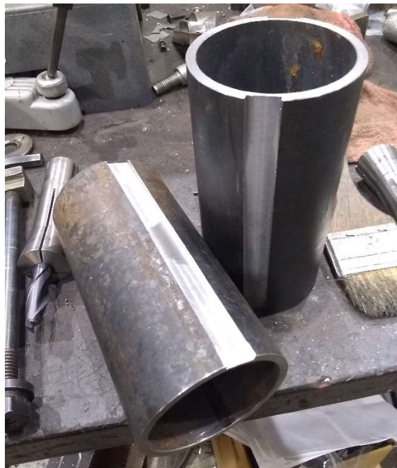
Figure 40. Finished outer drum grooves; backup and main
