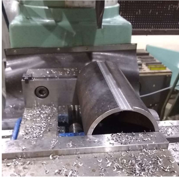
Figure 39. Drum, after milling first groove
