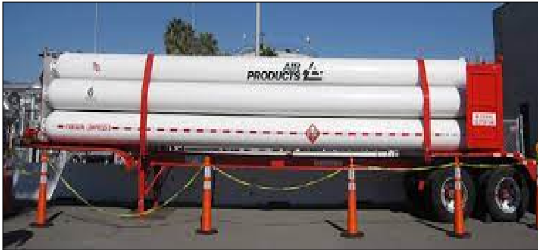
Figure 2-4: Gaseous Hydrogen Transportation Via Tube Trailer Trucks [14]
