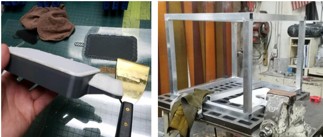
Figure 13 - Manufacturing Processes – 3-D printed piston (left) & frame tack welded in preparation for final welding (right)
