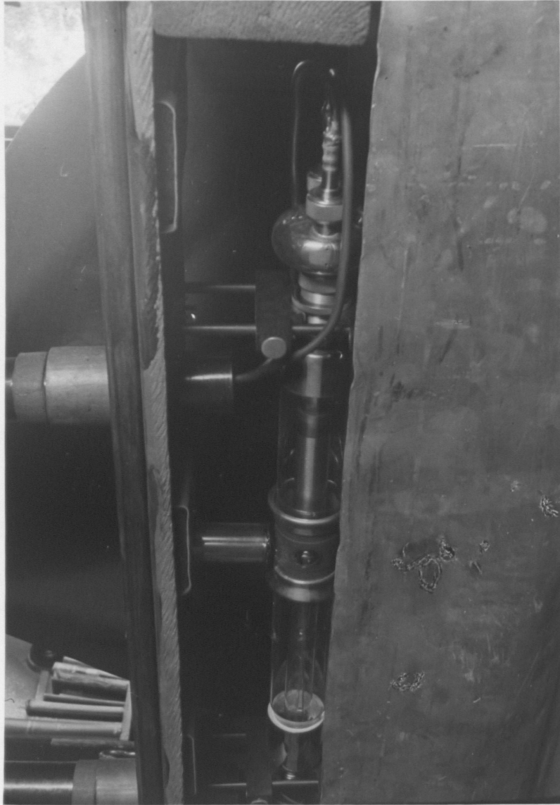
Fig. 8 View of X-ray tube before lowering it into tank.
