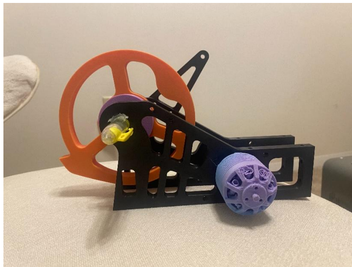
Figure 38: 3D-Printed Spinner Assembly
