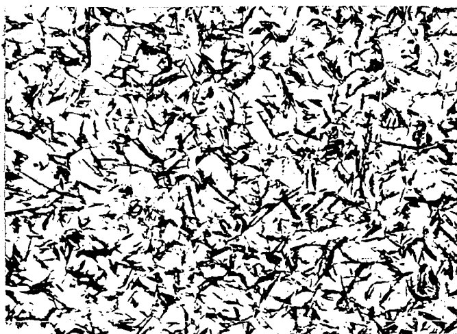
Fig. 16. Martensite formed on cooling 0.80% carbon to 186°C. Aust. Temp. 1050°C. 36% martensite. 300X
