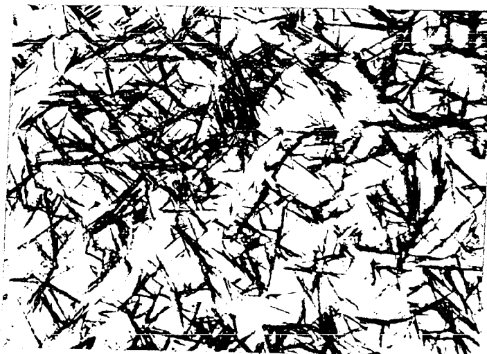
Fig. 30. 1.25% carbon steel isothermally transformed 33 minutes at 280°C. 15% Bainite 300X
