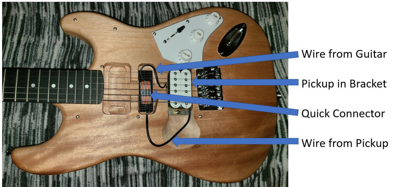
(Figure 21: The final build of the guitar with modular pickups)
