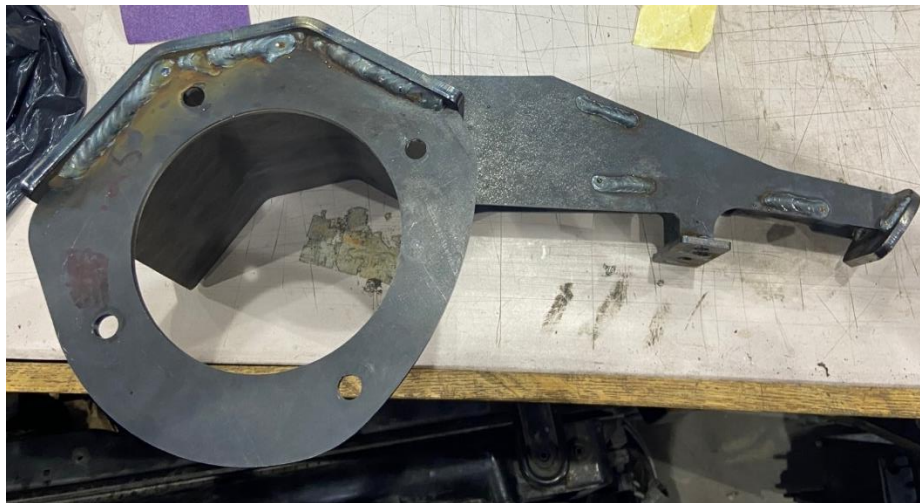
Figure 44 Motor Mount after Fabrication
