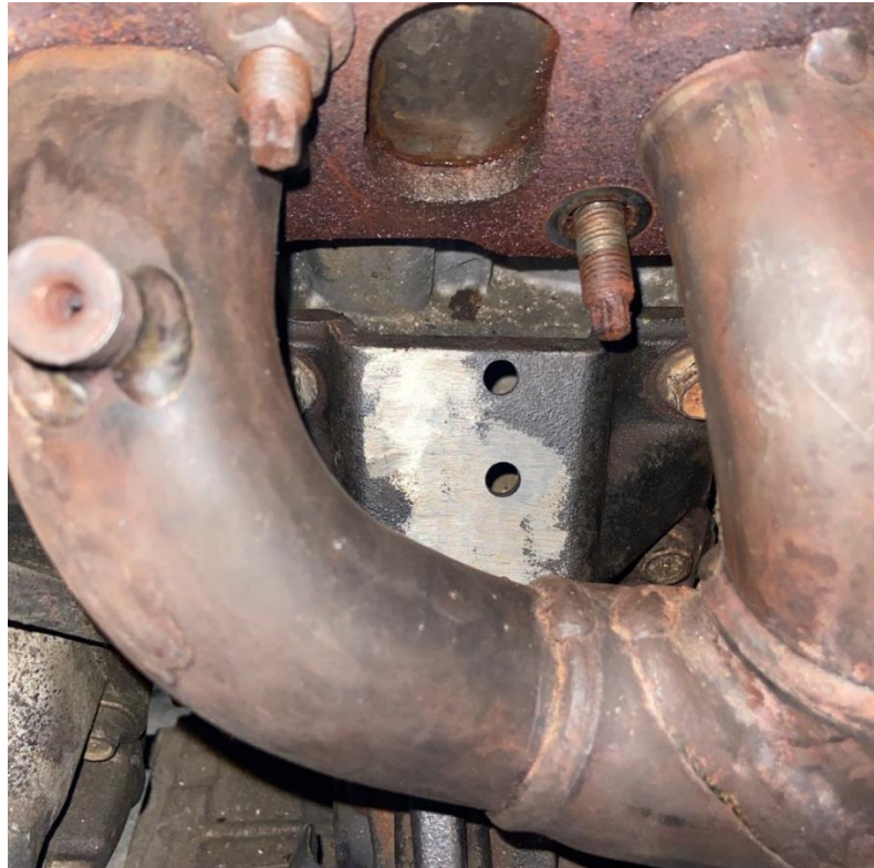
Figure 47 Engine Motor Mounted after Drilled and Installed
