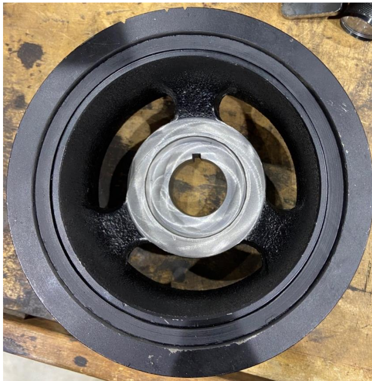
Figure 51 Machined Harmonic Balancer
