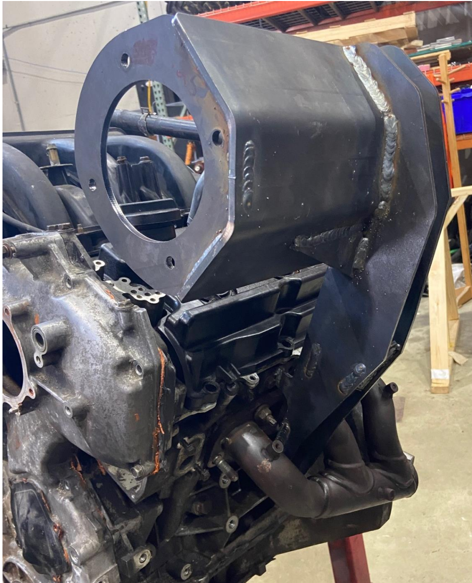
Figure 46 Motor Mount mounted of Mock Block
