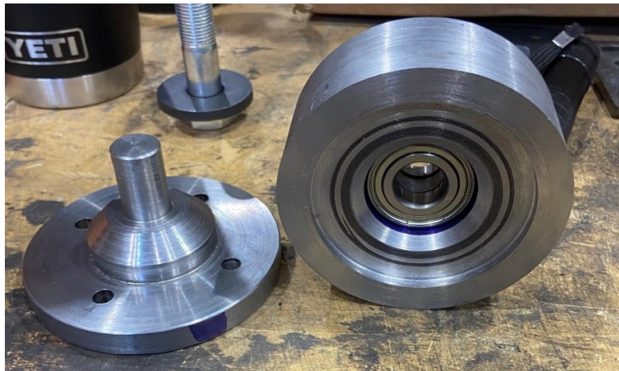
Figure 48 Machined Components for Idler Pulley
