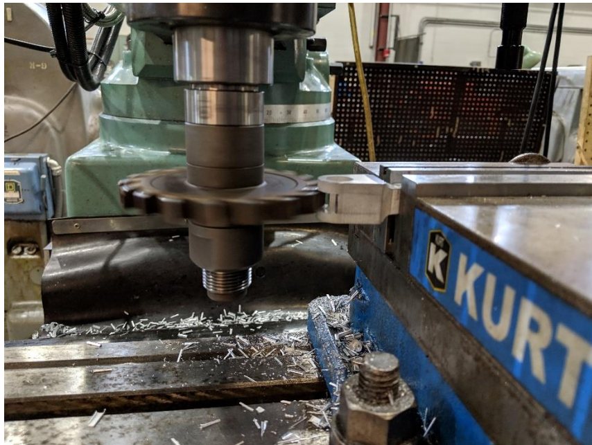
Figure 12: Slot Being Cut into the A-Arm
