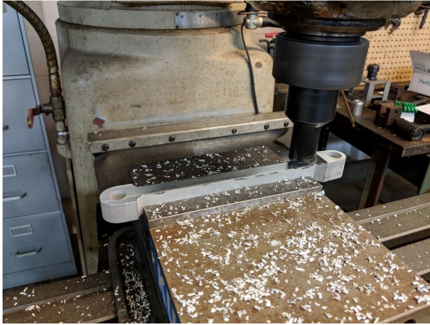
Figure 11: Machining of the A-arm
