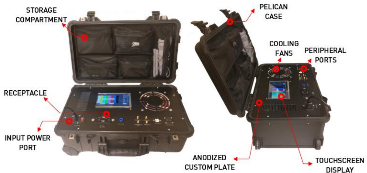
Figure 1: Completed Mission Box
