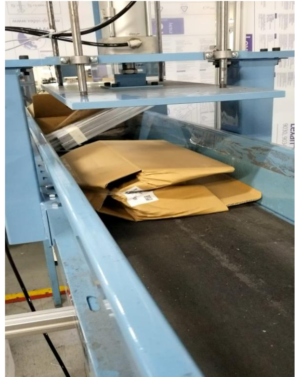
Figure 25: Crushed box from a side orientation
