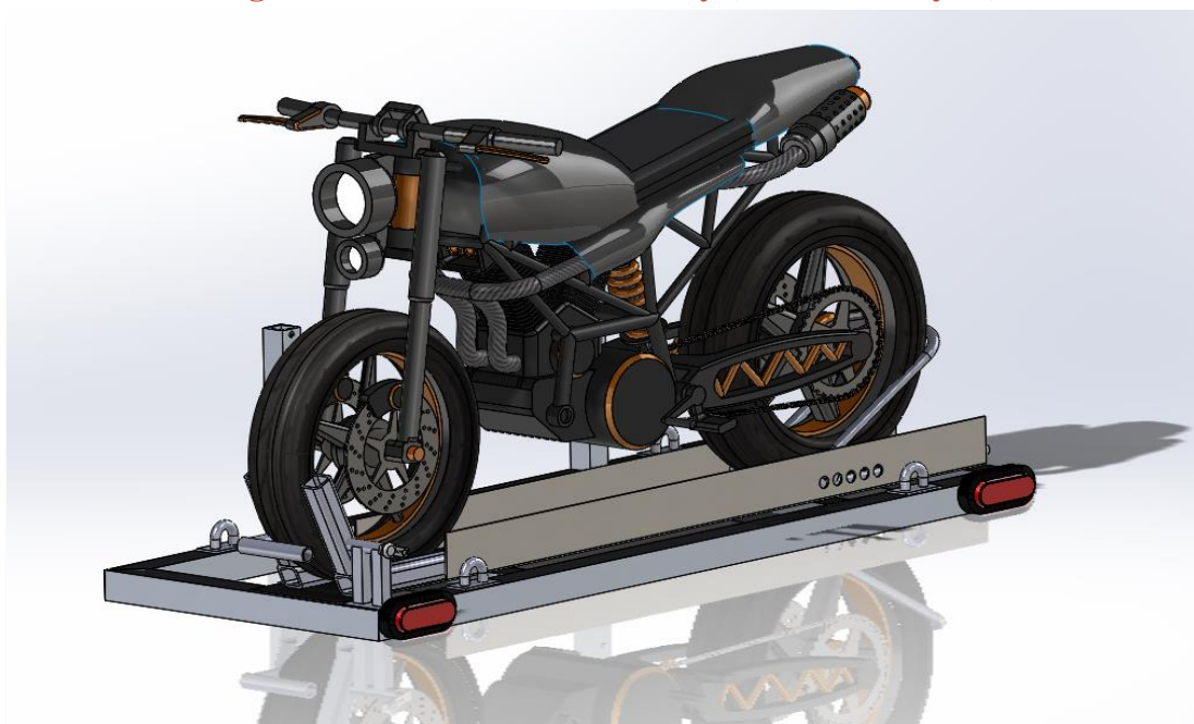
Figure 27: Final Frame Assembly (With Motorcycle)
