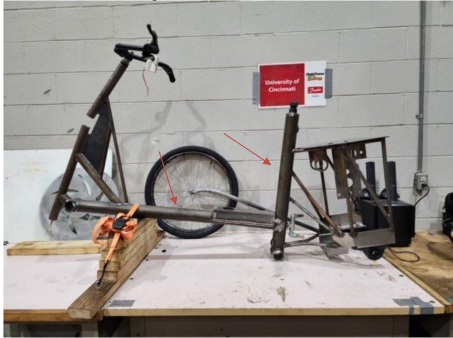
Figure 10: Hydraulic Tank as Part of the Frame
