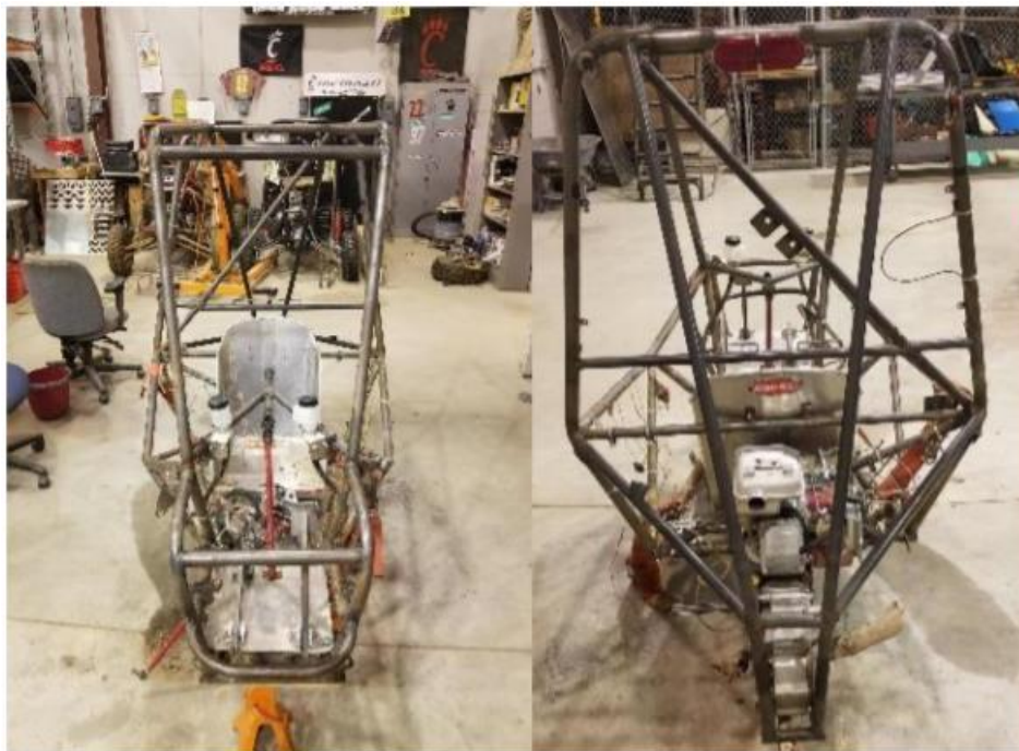
Figure 5: 2018 UC Baja Car Roll Cage [5]
