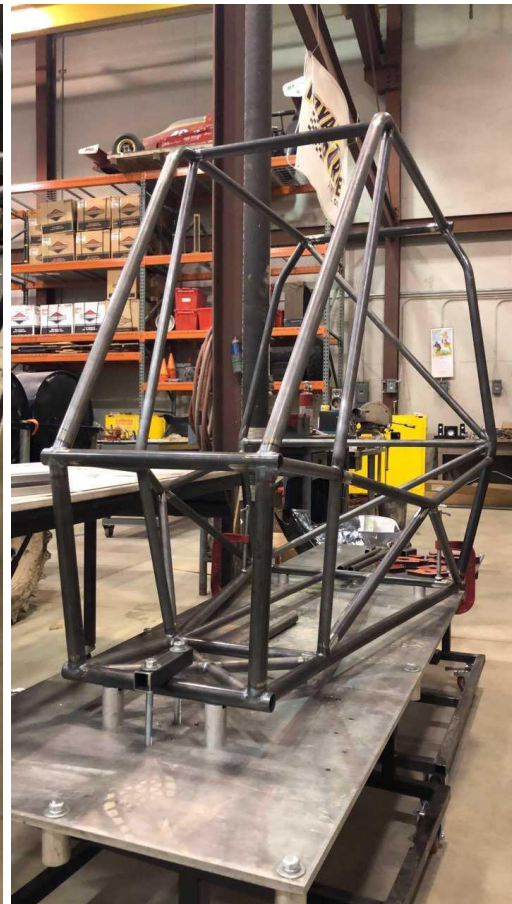
Figure 18 - Completed Frame in Jig
