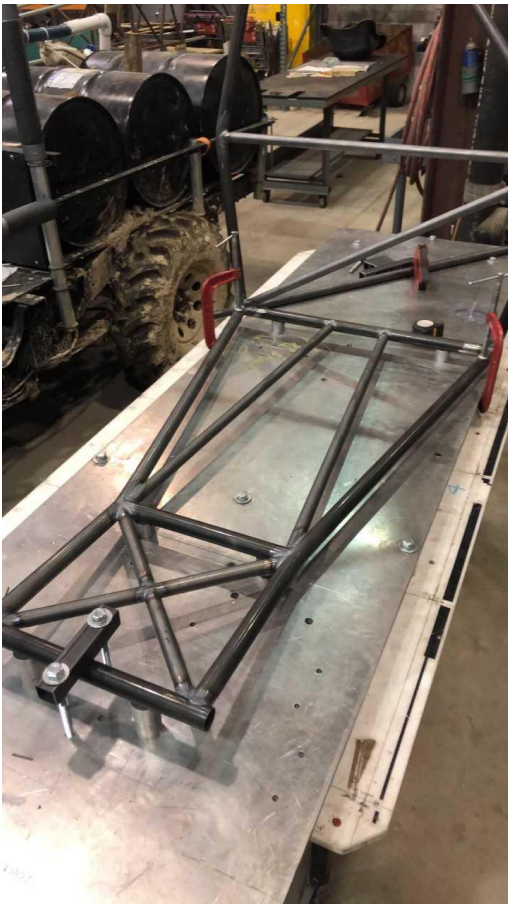
Figure 17 - Base Frame in Jig
