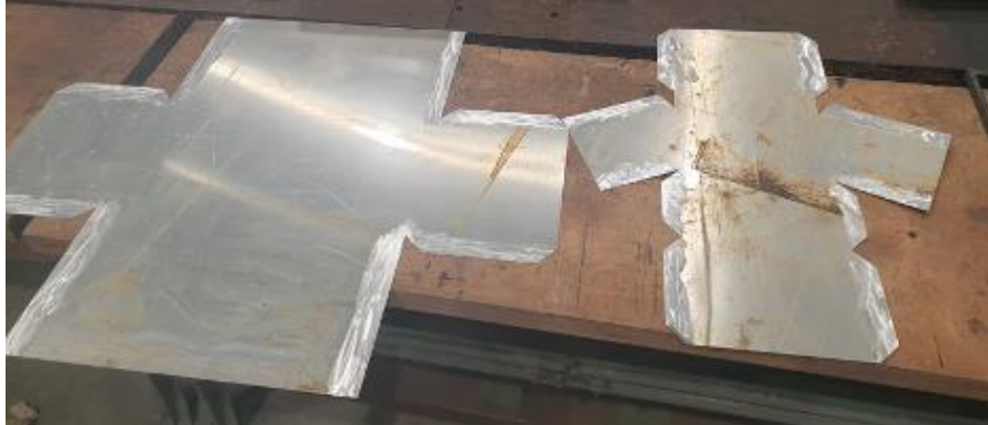
Figure 49 – Cut Sheet Metal for Cabs
