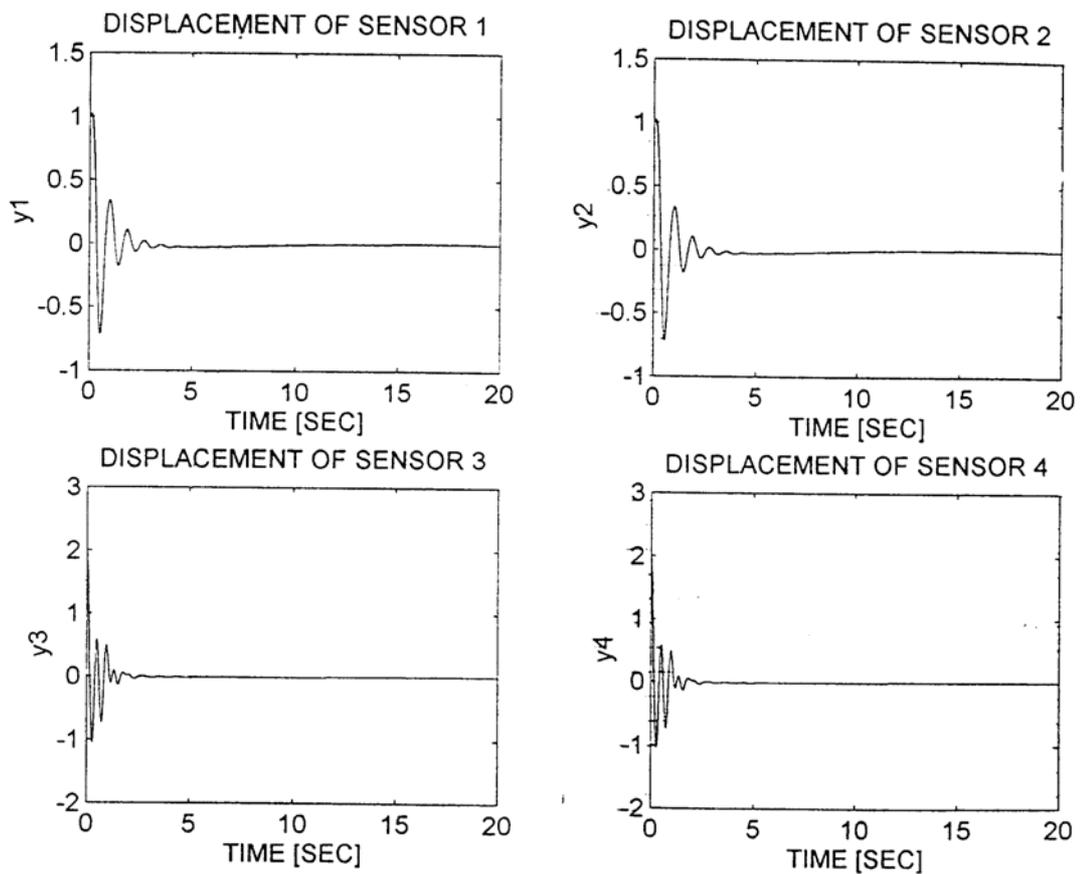
Figure 4: Closed-loop response using fuzzy based strategy.
