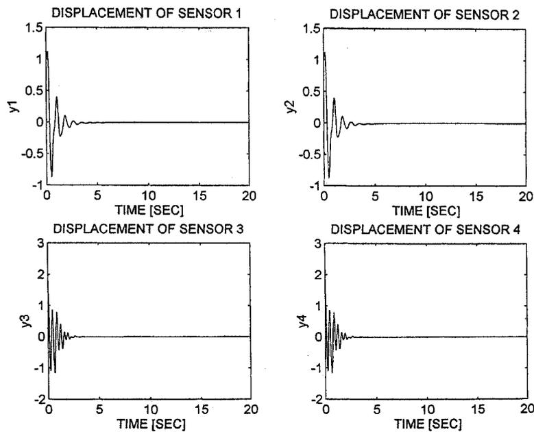
**Figure 13.** Robustness test for initial condition using adaptive fuzzy controller—case 2 for the four sensors.
