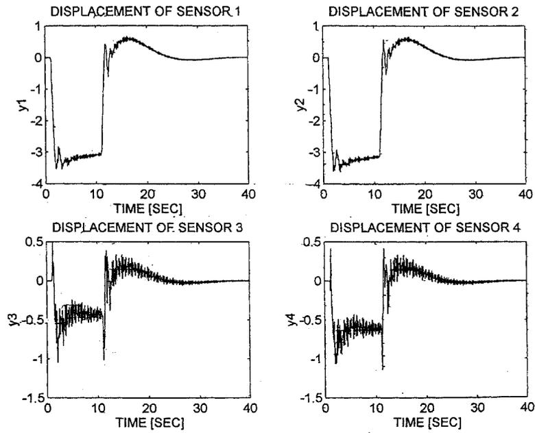
Figure 10. Robustness test using adaptive fuzzy controller—case 3 for the four sensors.
