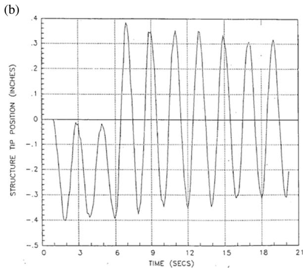
**Figure 4.** Open-loop response of the structure tip for a persistent pulse: (a) present study, (b) Parlos and Jayasuriya (1990).
