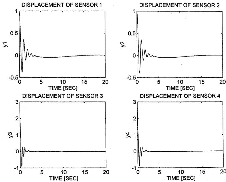
**Figure 12.** Robustness test for initial condition using adaptive fuzzy controller—case 1 for the four sensors.
