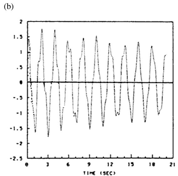
**Figure 5.** Open-loop response of the structure tip for an initial condition: (a) present study, (b) Lynch and Banda (1988).
