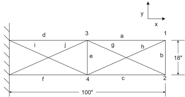
Figure 3. AFWAL/FIB 10 bar truss (Lynch and Banda 1988).
