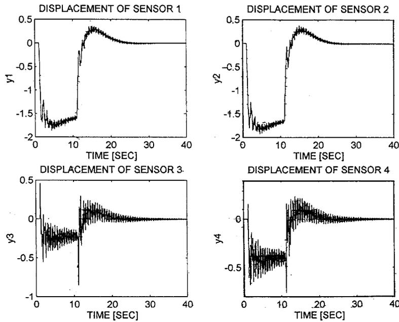
Figure 9. Robustness test using adaptive fuzzy controller—case 2 for the four sensors.
