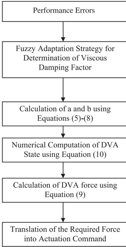
Figure 2. Calculation of actuation command.
