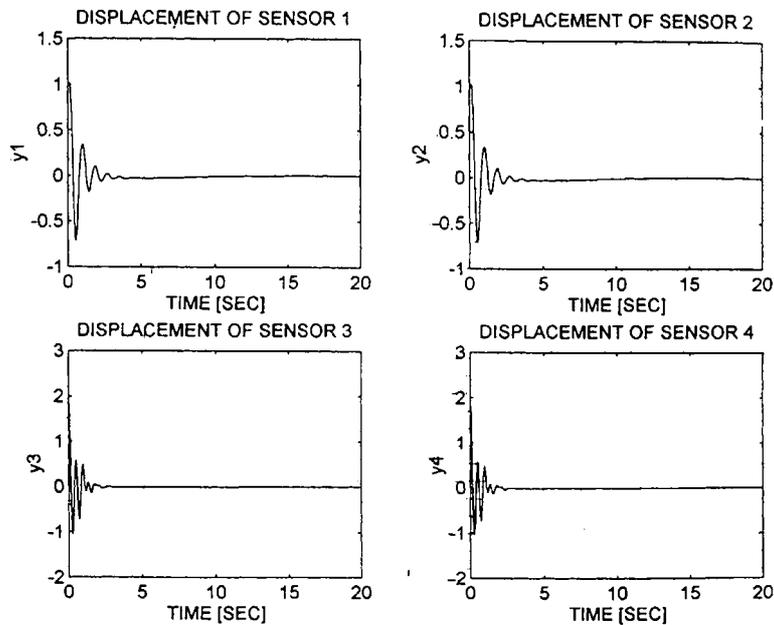
Figure 11. Transient response to initial condition using LQG/LTR control for the four sensors.
