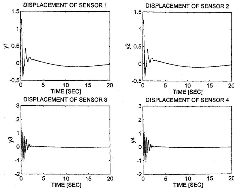
**Figure 14.** Robustness test for initial condition using adaptive fuzzy controller—case 3 for the four sensors.
