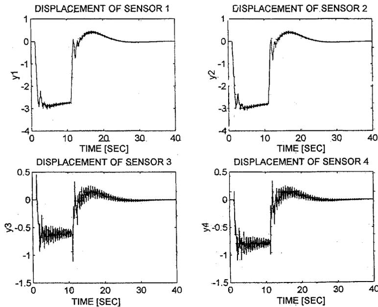
Figure 8. Robustness test using adaptive fuzzy controller—case 1 for the four sensors.
