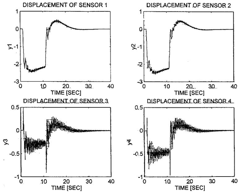
Figure 7. Transient response to persistent disturbance using adaptive fuzzy controller for the four sensors.
