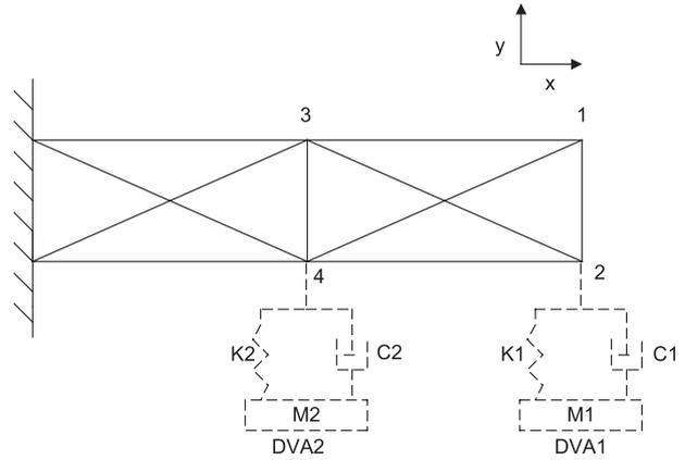
**Figure 6.** Application of two virtual DVAs to the 10 bar truss.
