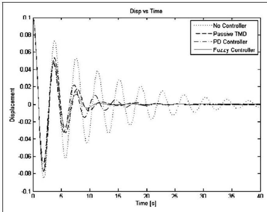
Figure 4. One story structure subject to initial displacement.
