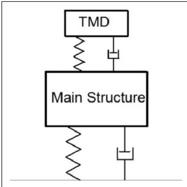
**Figure 1.** Schematic diagram of a tuned mass damper attached to the main structure.
