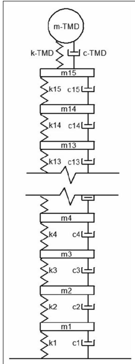
**Figure 6.** Schematic diagram of the 15 story structure with tuned mass damper attached to it.
