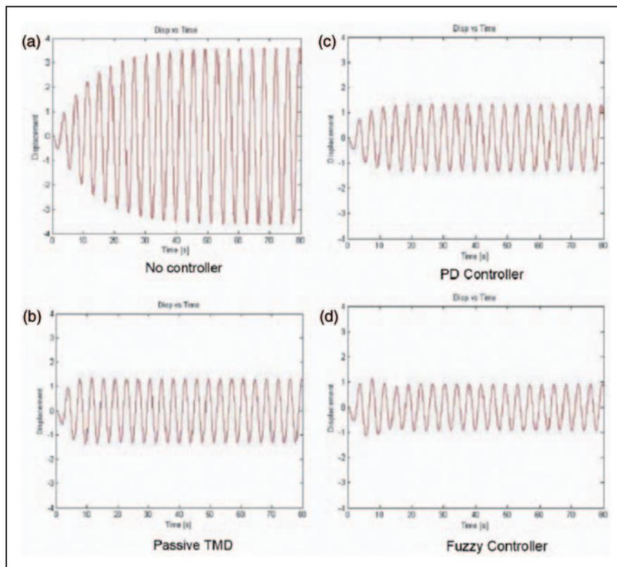
**Figure 5.** One story structure subject to forced harmonic vibration.
