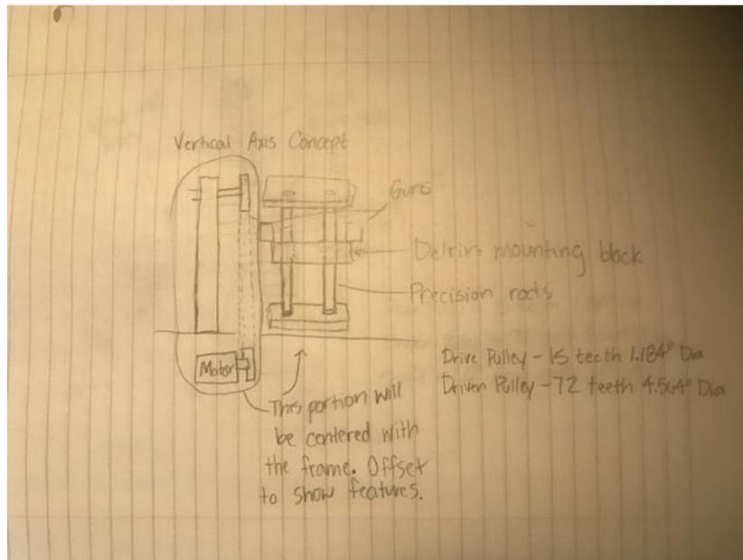
Figure 4 - Vertical Axis Concept Design
