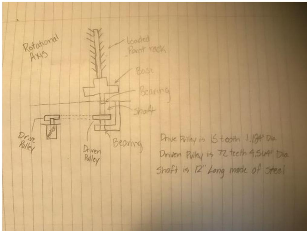
Figure 5 - Rotational Axis Concept Design
