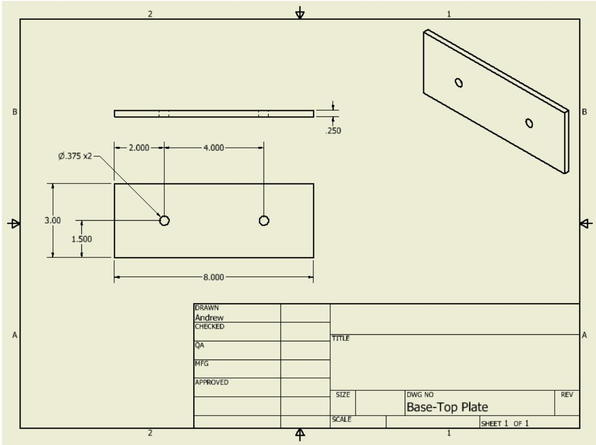
Figure 18 - Top and Bottom Support Plates
