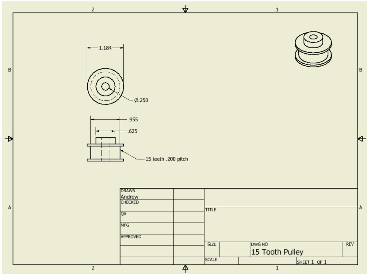
Figure 16 - Drawing for 15 Tooth Drive Pulley
