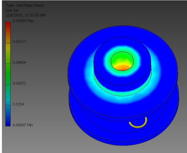
Figure 8 - FEA Analysis of Drive Pulley for Vertical Axis
