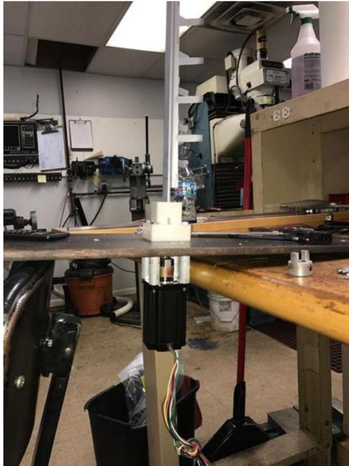
Figure 24 - Rotational Axis Assembly
