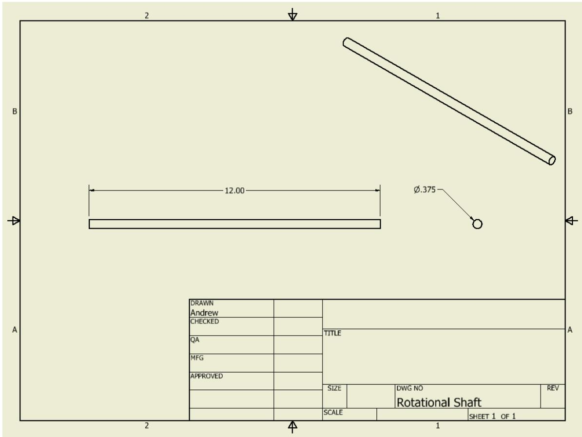
Figure 20 - Shaft for Rotational Axis
