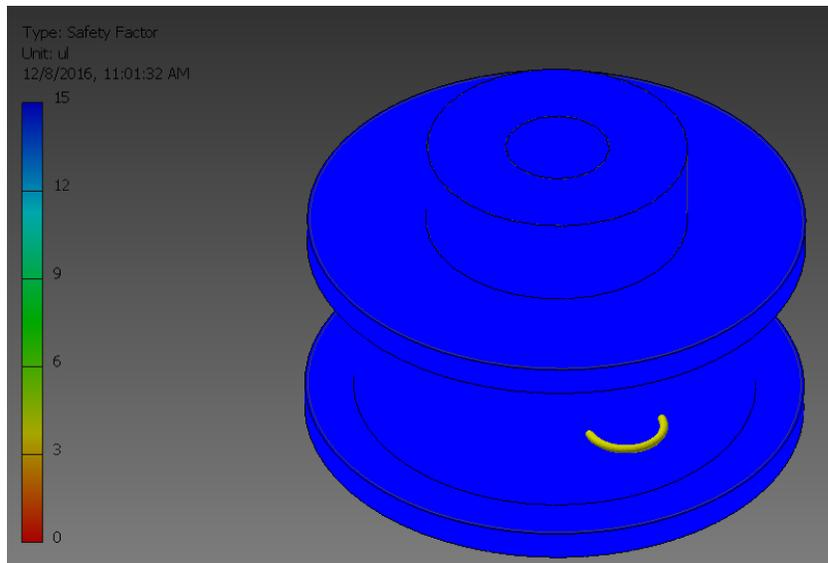
Figure 11- Safety Factor of Drive Pulley for Rotational Axis
