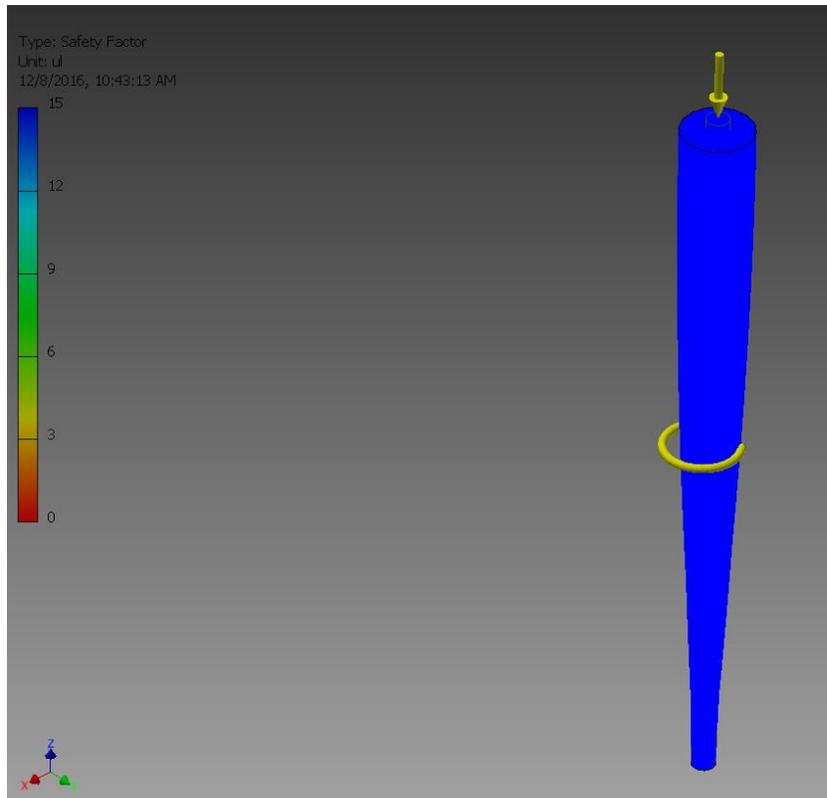
Figure 13 - Safety Factor of Driven Shaft for Rotational Axis
