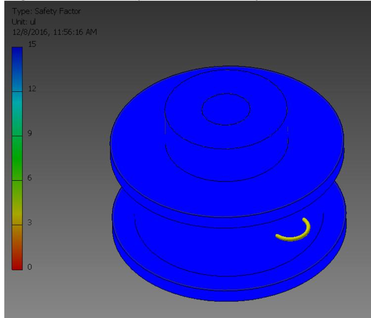
Figure 9 - Safety Factor of Drive Pulley for Vertical Axis
