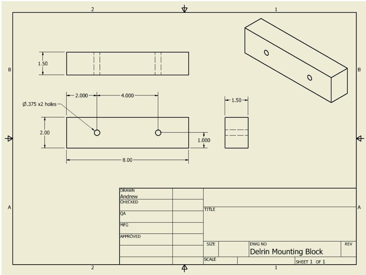
Figure 19 - Delrin Mounting Block
