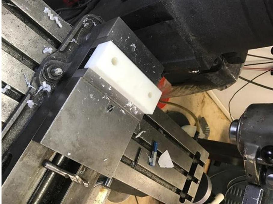
Figure 22 - Delrin Mounting Block
