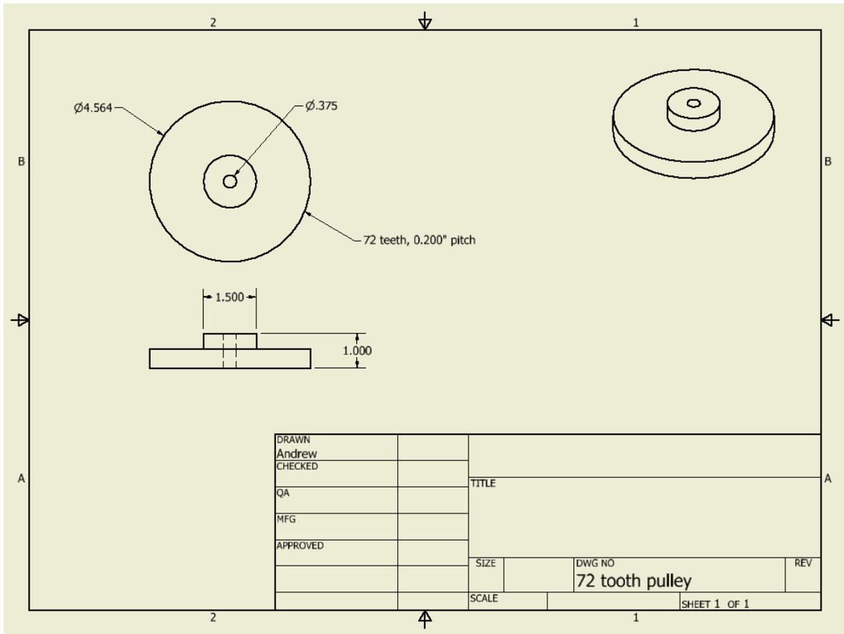
Figure 17 - Drawing for 72 Tooth Driven Pulley
