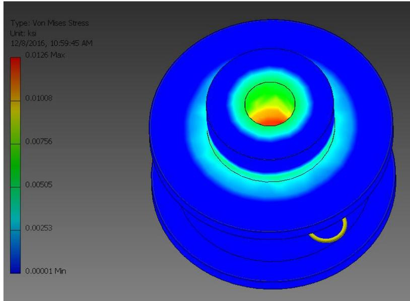
Figure 10 - FEA Analysis of Drive Pulley for Rotational Axis
