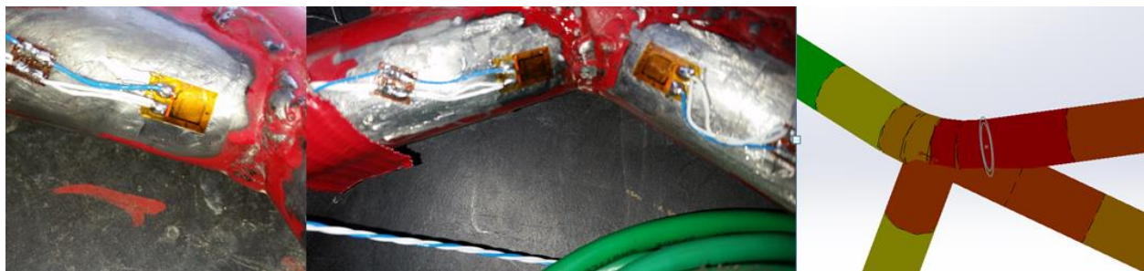
Figure 11 – Demonstration of strain gauge size vs FEA element size
