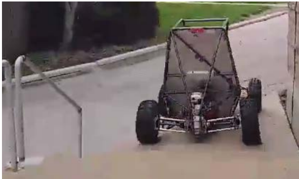
Figure 30 - 3ft Drop Test
