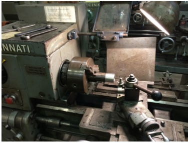
Figure 24 - Turning material on lathe
