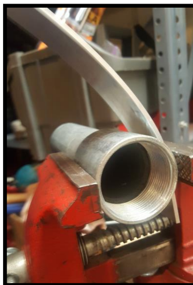
Figure 13: U Bracket Fabrication
