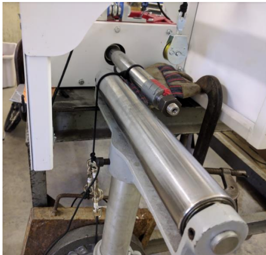
Figure 101: x-axis Validation Setup with Support Roller Stand
