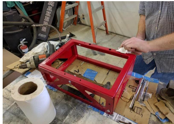
Figure 77: Cleaning LC Cage Drill Debris
