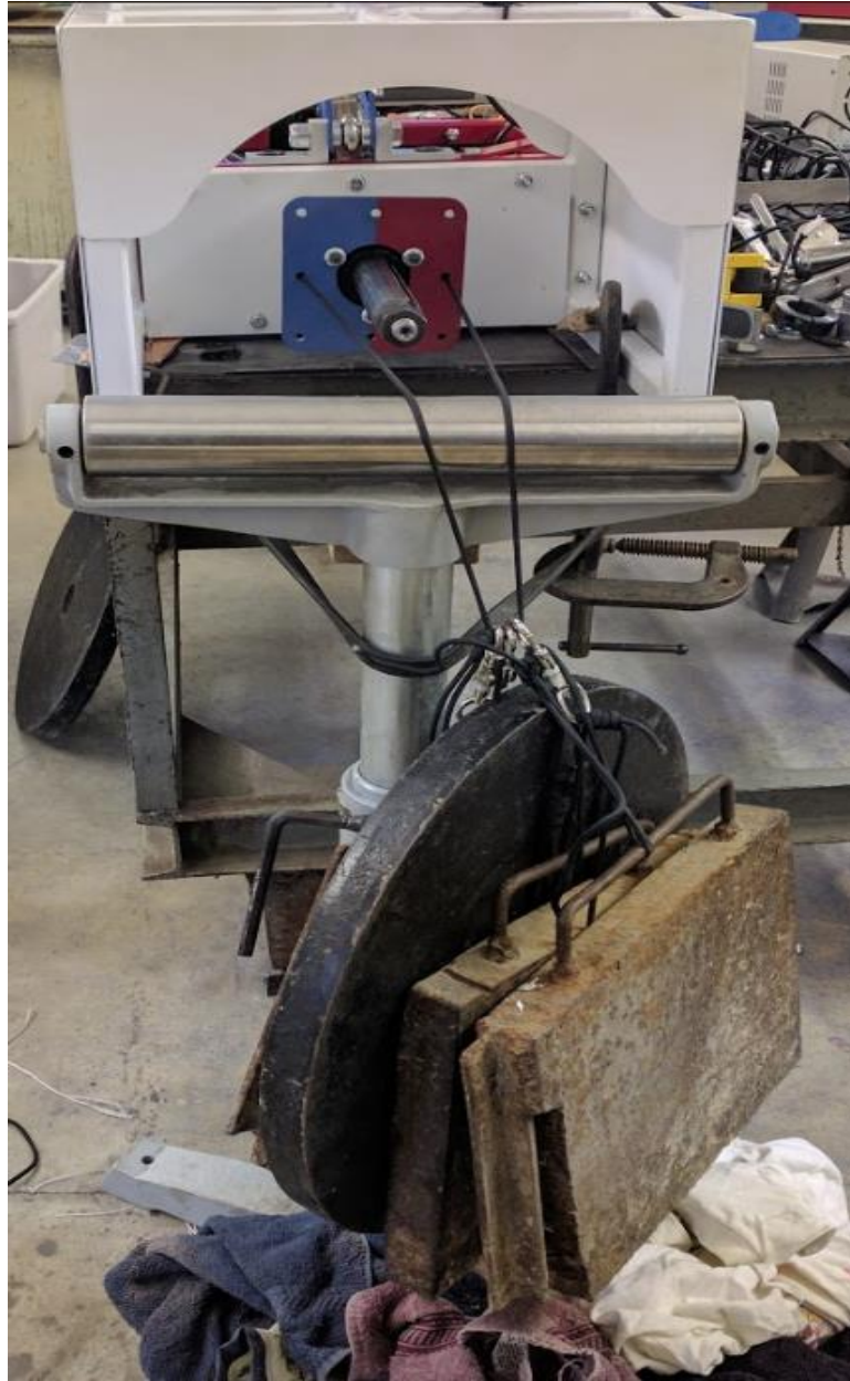
Figure 103: y-axis Validation Setup with Support Roller Stand
