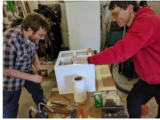
Figure 75: Tire Cage Drilling
