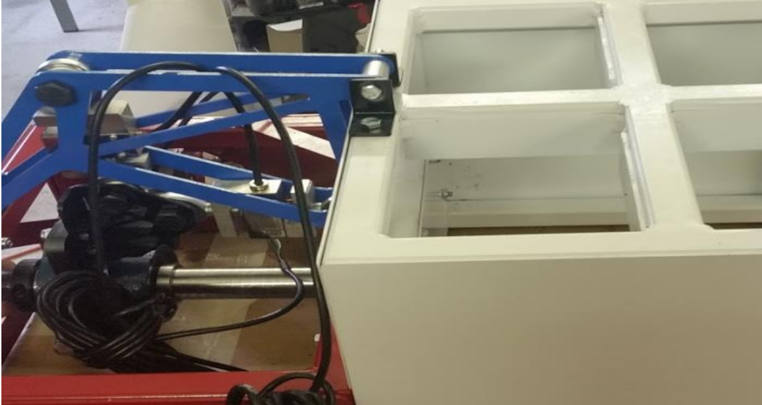
Figure 90: Fitting Vertical Support Brackets to Tire Cage
