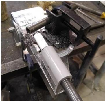
Figure 11: Tube notching setup
