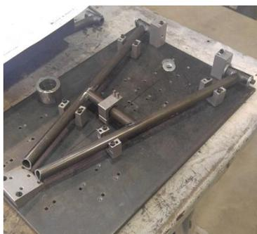
Figure 12: Welding Jig
