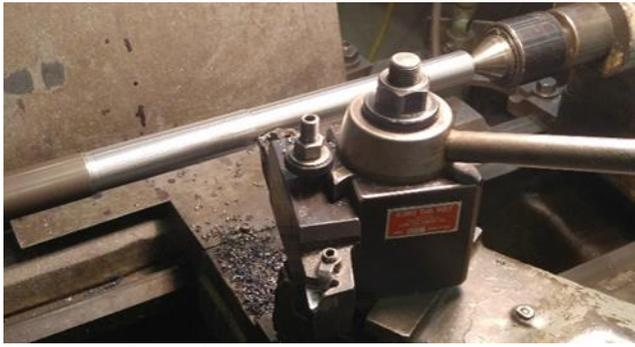
Figure 14: Threaded insert lathe setup
