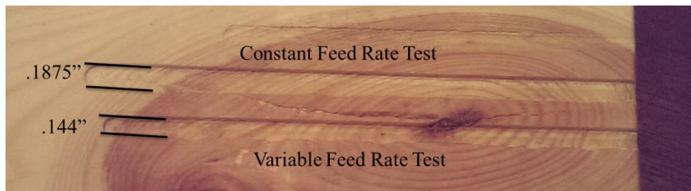
Figure 26: Impact Deflection Test Results
