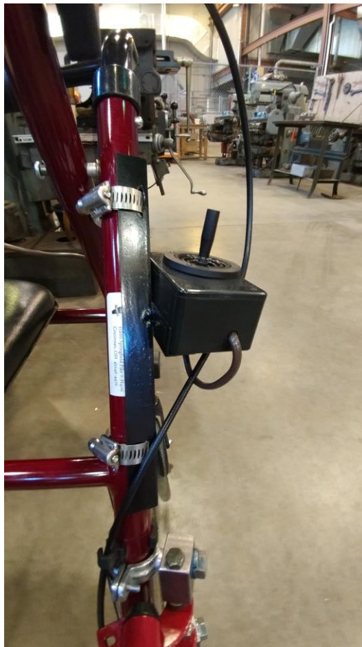
Figure 27: Joystick Mount Assembled to Walker
