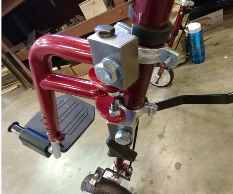
Figure 22: Footrest Mount Assembly (side view)
