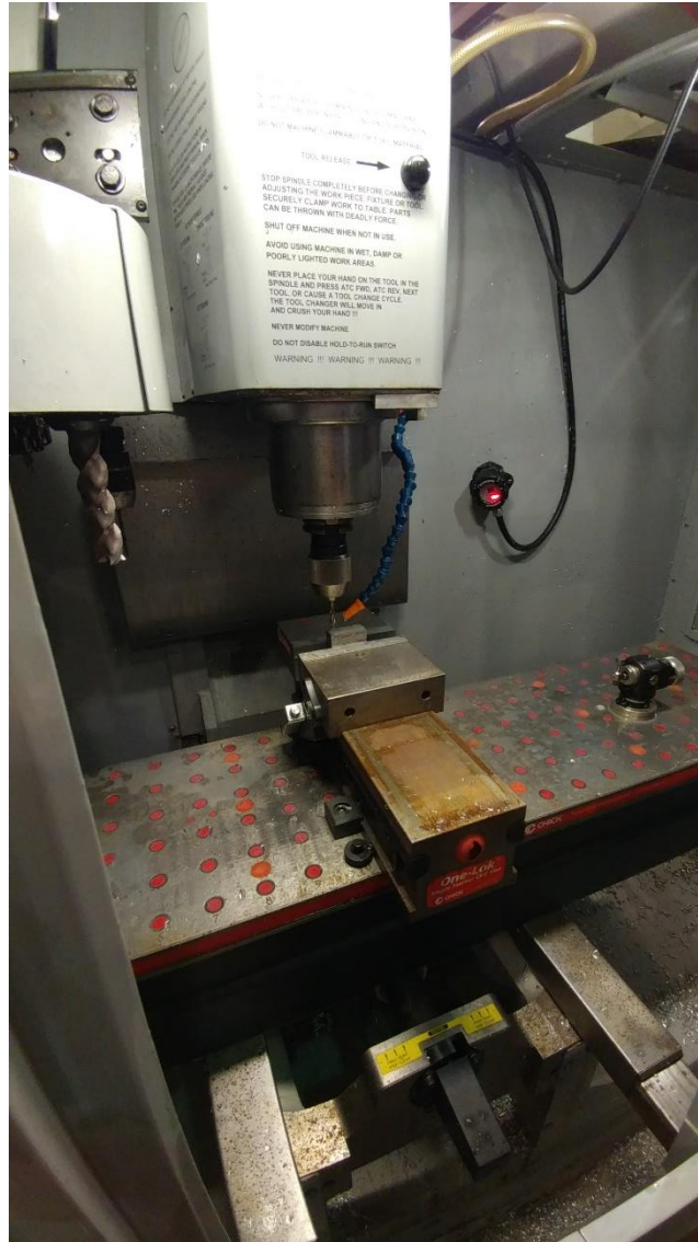
Figure 20: Footrest mount after 1/4"-20 holes have been drilled
