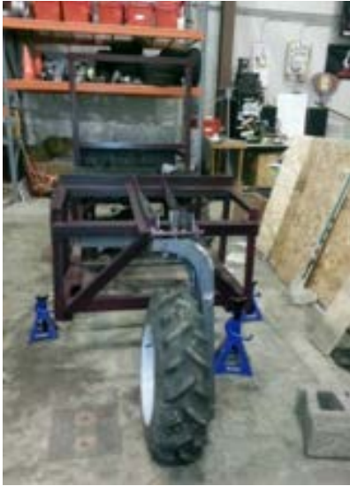
Figure 23: Fabrication – Chassis to Front Suspension
