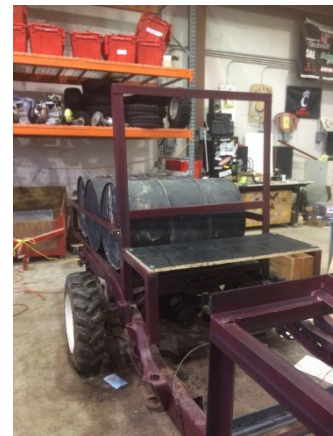
Figure 22: Fabrication - Completed Cargo Bed
