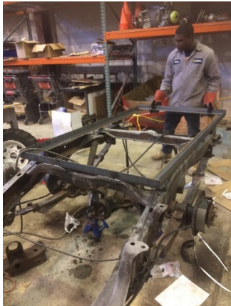
Figure 21: Fabrication - Cargo Bed in Progress
