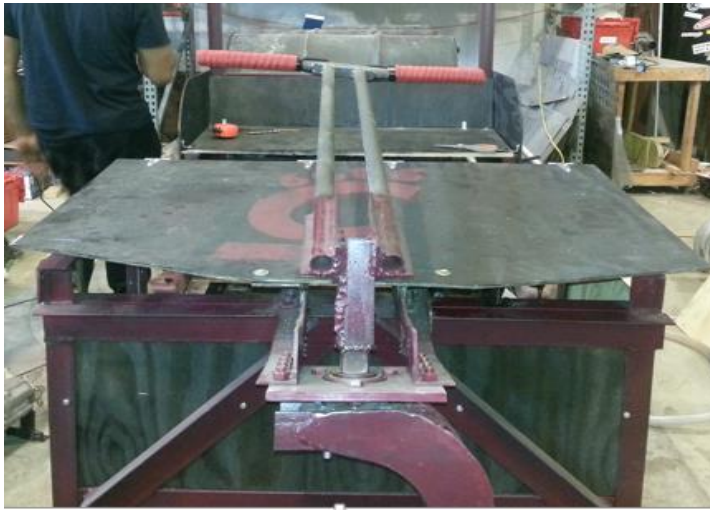
Figure 17: Steering mounted onto front suspension
