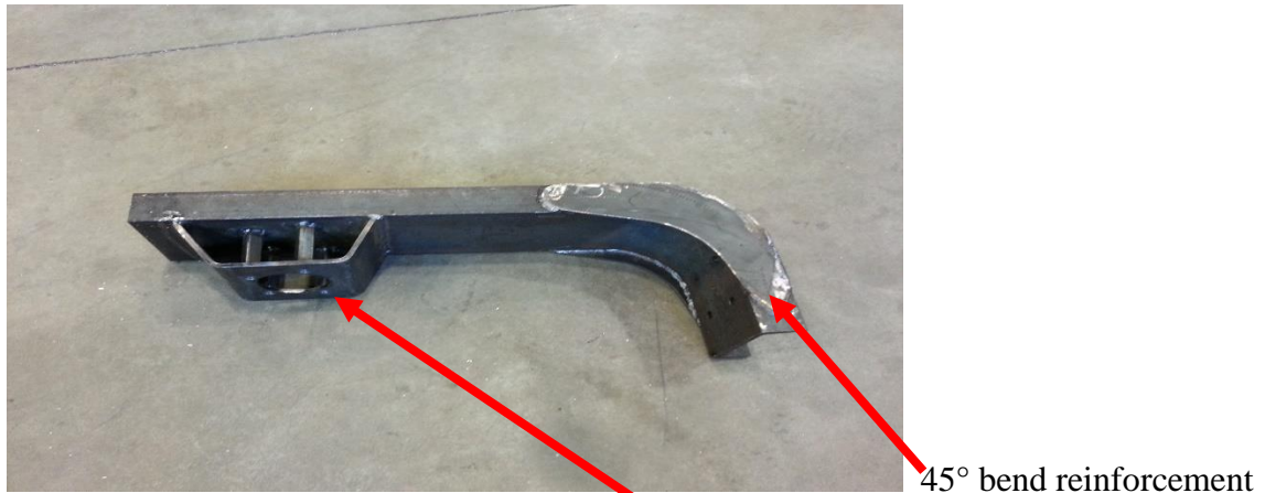
Figure 13: Welding and fabrication of suspension Wheel hub mount (female for hub)
