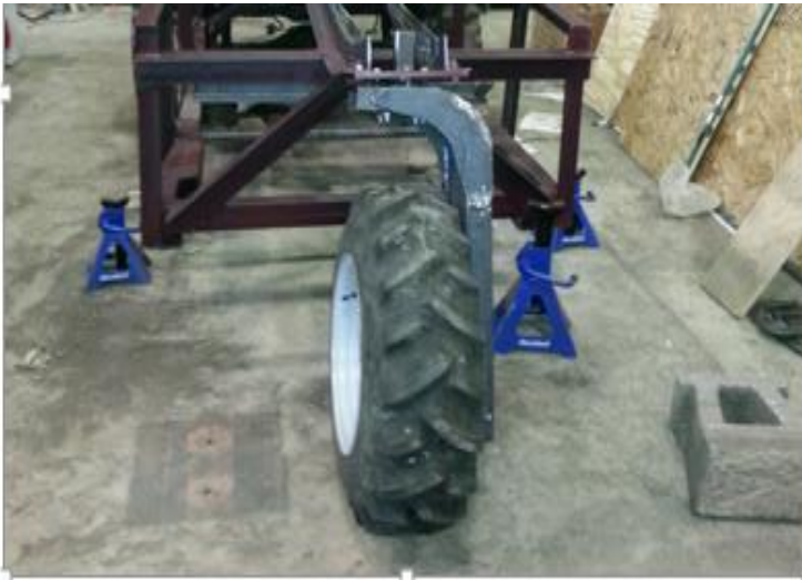
Figure 16: Assembly of Unit-Strut front suspension
