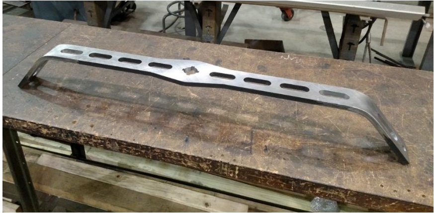
Figure 13-Weapon Blade Before Heat Treatment
