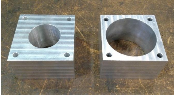
Figure 19-Weapon Bearing Block Before and After Turning
