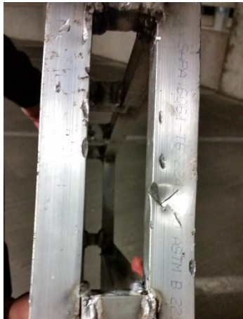
Figure 29--Dents and Holes in Target Frame
