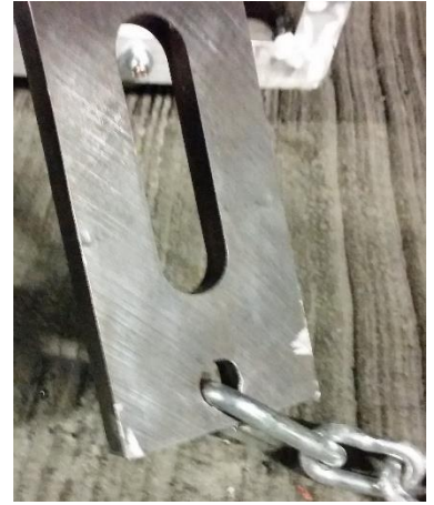
Figure 31-Cosmetic Damage on Blade
