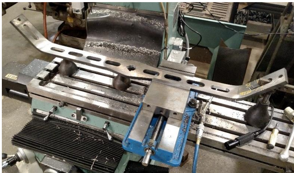
Figure 22-Weapon Blade Final Machining Before Heat Treatment
