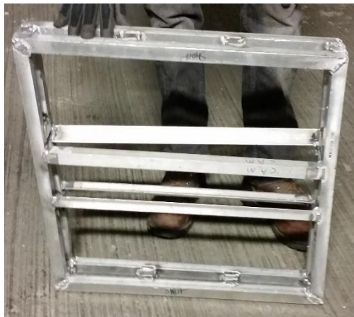
Figure 30-Target Frame, Multiple Weld Failure
