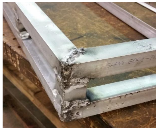
Figure 8-Corner of test frame from practical drop test
