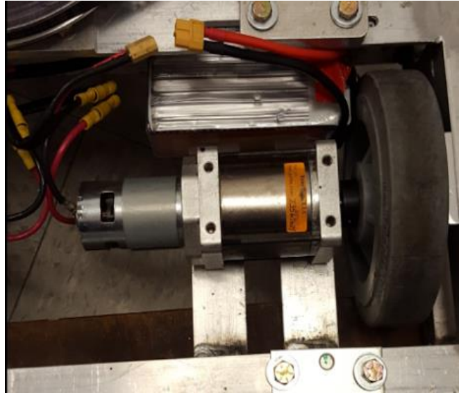
Figure 24-Installed Motor and Wheel Assembly
