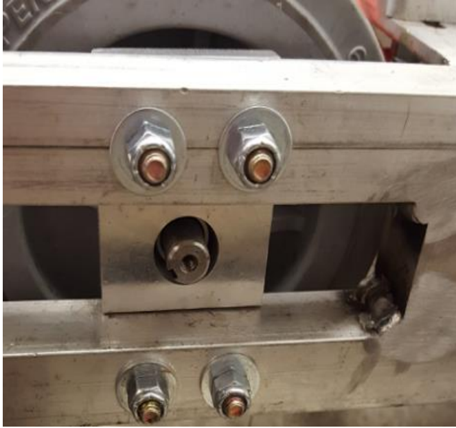
Figure 26-Installed Drivetrain Bearing Block
