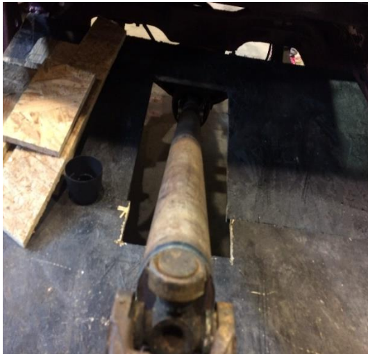
Figure 13: Driveshaft connected to transmission
