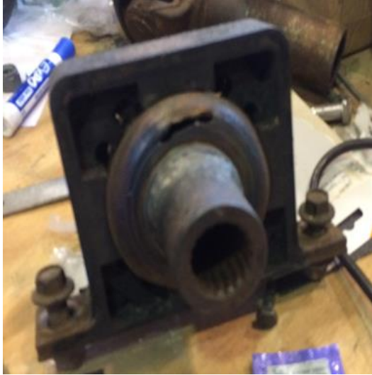
Figure 12: Manufactured coupler shaft
