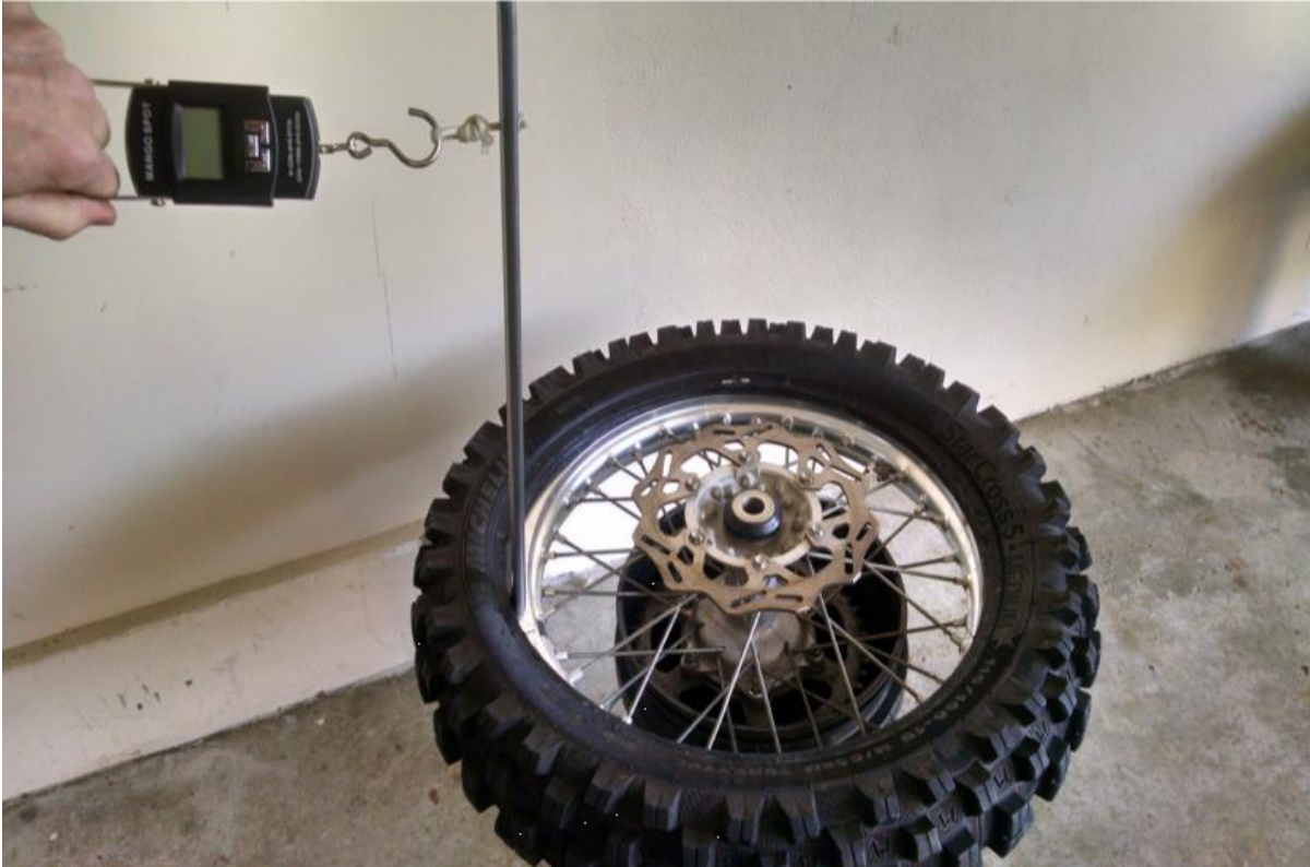
Figure 8 Apparatus for testing loads during a tire change
