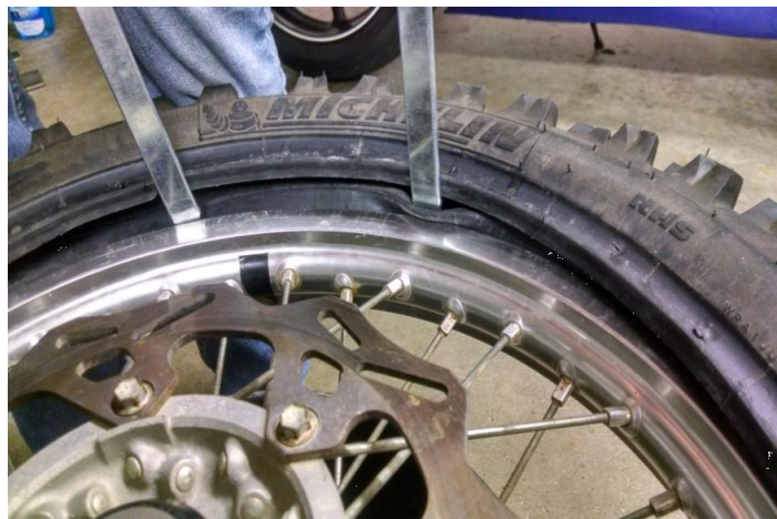
Figure 1 Visual representation of a pinch flat. Note that this example is exaggerated for clarity
