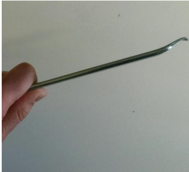
Figure 3 Profile of Tire Spoon. The hooked end is used to grab the aluminum rim
