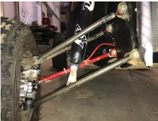
Figure 17: The tie rod is shown in red. This gives an idea of the tie rod alignment and location in relation to the suspension arms to prevent bump steer.
