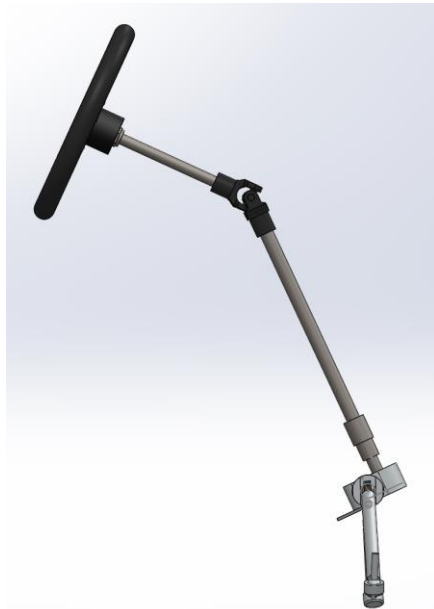
Figure 6: New steering column with one U joint, rather than two.
