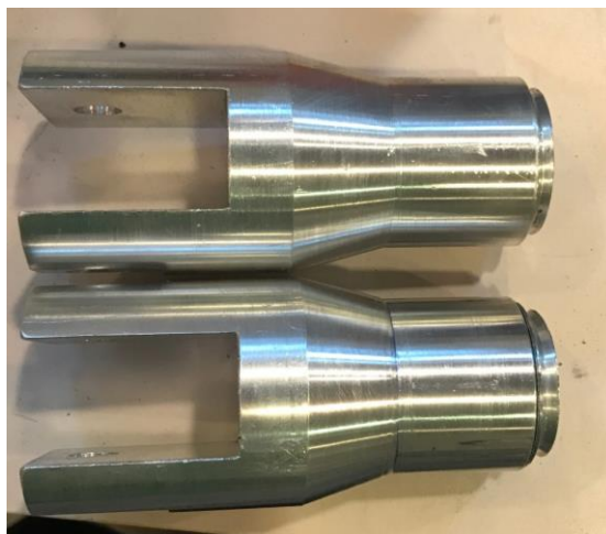
Figure 14: This is a picture of the two rack extensions after the machining operations have been completed.
