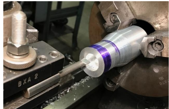
Figure 13: This picture shows the hole being bored into the end of the rack extension. The tool used for this operation was a boring bar.
