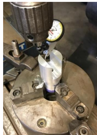
Figure 14: This figure shows the fixturing for the end milling operations.
