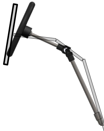
Figure 1: The new design is shown in darker grey and black. The lighter grey model shows the 2014 steering column shape.
