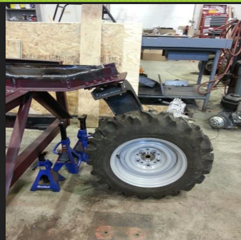
Front tire mounted onto suspension
