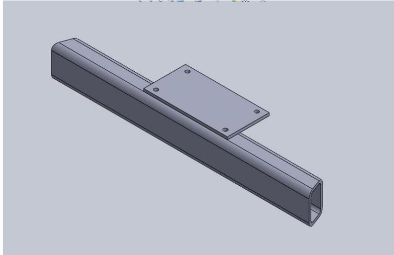
Figure 9: Winch mount modeled in Solidworks
