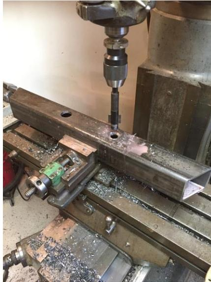
Figure 24: Drilling the access holes
