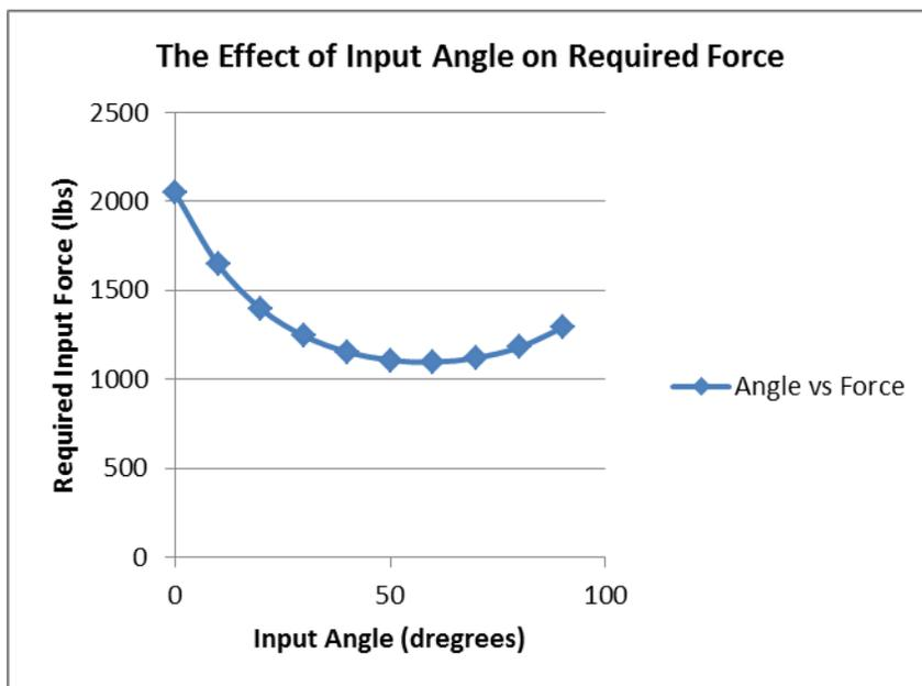
Figure 1: Effect of Input Angle of Required Force
