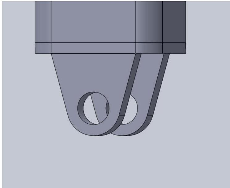
Figure 3: Detail of the end cap and mounting tab configuration.
