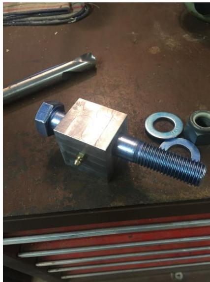
Figure 19: Hinge blocks test fitted for hinge pin and grease fitting
