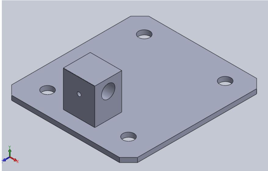
Figure 7: Hinge Plate modeled in Solidworks
