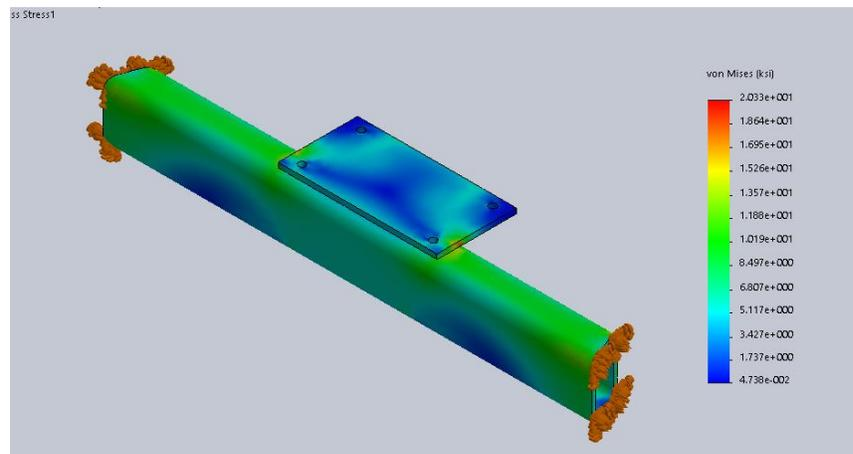
Figure 10: FEA results for the winch mount
