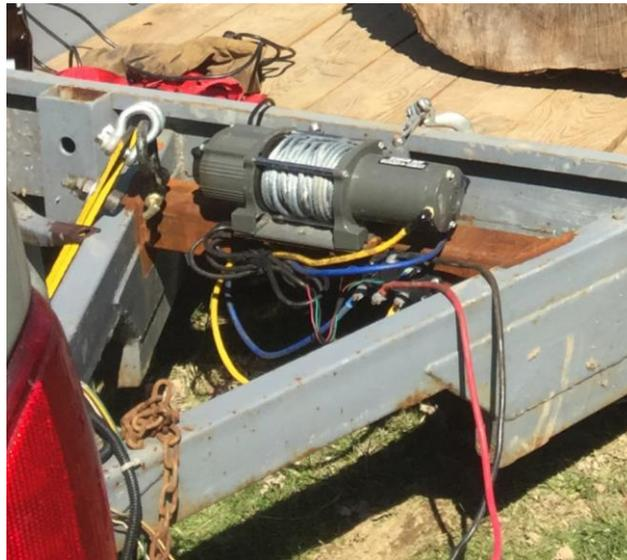
Figure 25: Complete winch installation on the trailer
