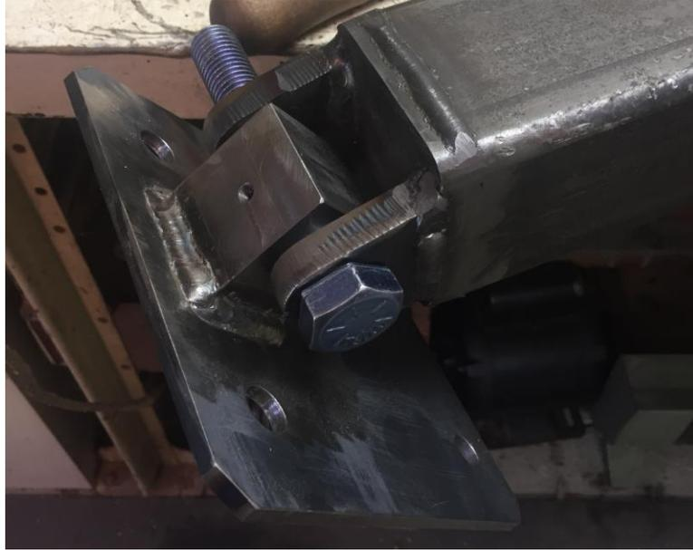
Figure 22: Test fitting the hinge joint
