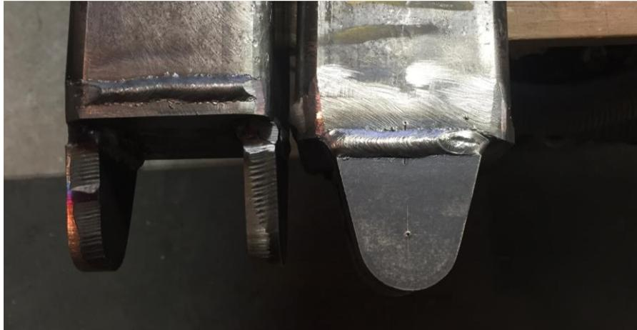
Figure 15: Mounting tabs fully welded on
