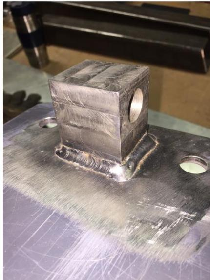
Figure 21: Hinge block welded to the plate
