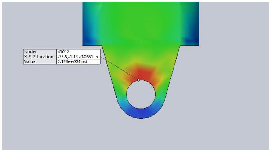
Figure 6: Maximum stress experienced by the mounting tabs
