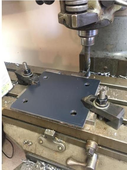
Figure 20: Hinge plate during drilling process
