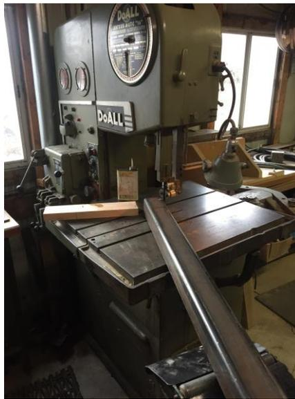
Figure 11: Cutting tubing to length using the band saw
