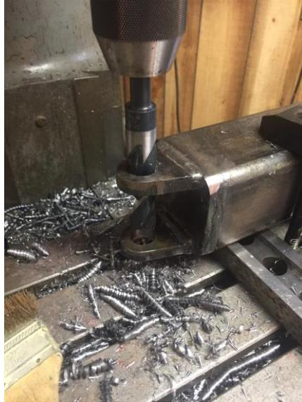
Figure 16: Drilling the holes in the mounting tabs simultaneously
