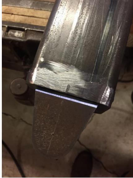
Figure 14: Locating the mounting tabs for welding
