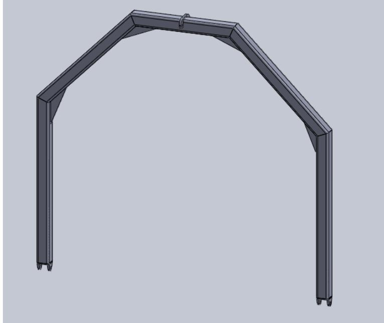
Figure 2: Lifting Arch as modeled in Solidworks
