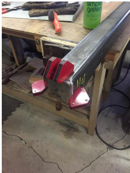
Figure 13: Fixturing the end cap for welding
