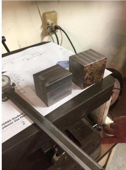
Figure 18: Hinge blocks midway through machining
