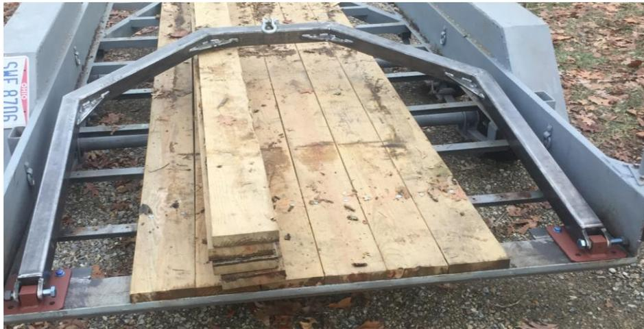
Figure 17: The completed lifting arch
