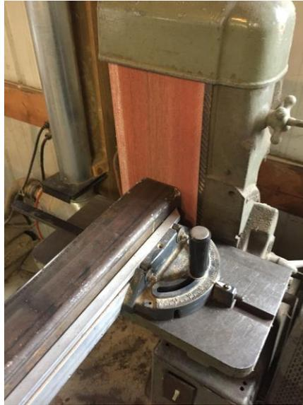
Figure 12: Sanding tubing accurately to dimension
