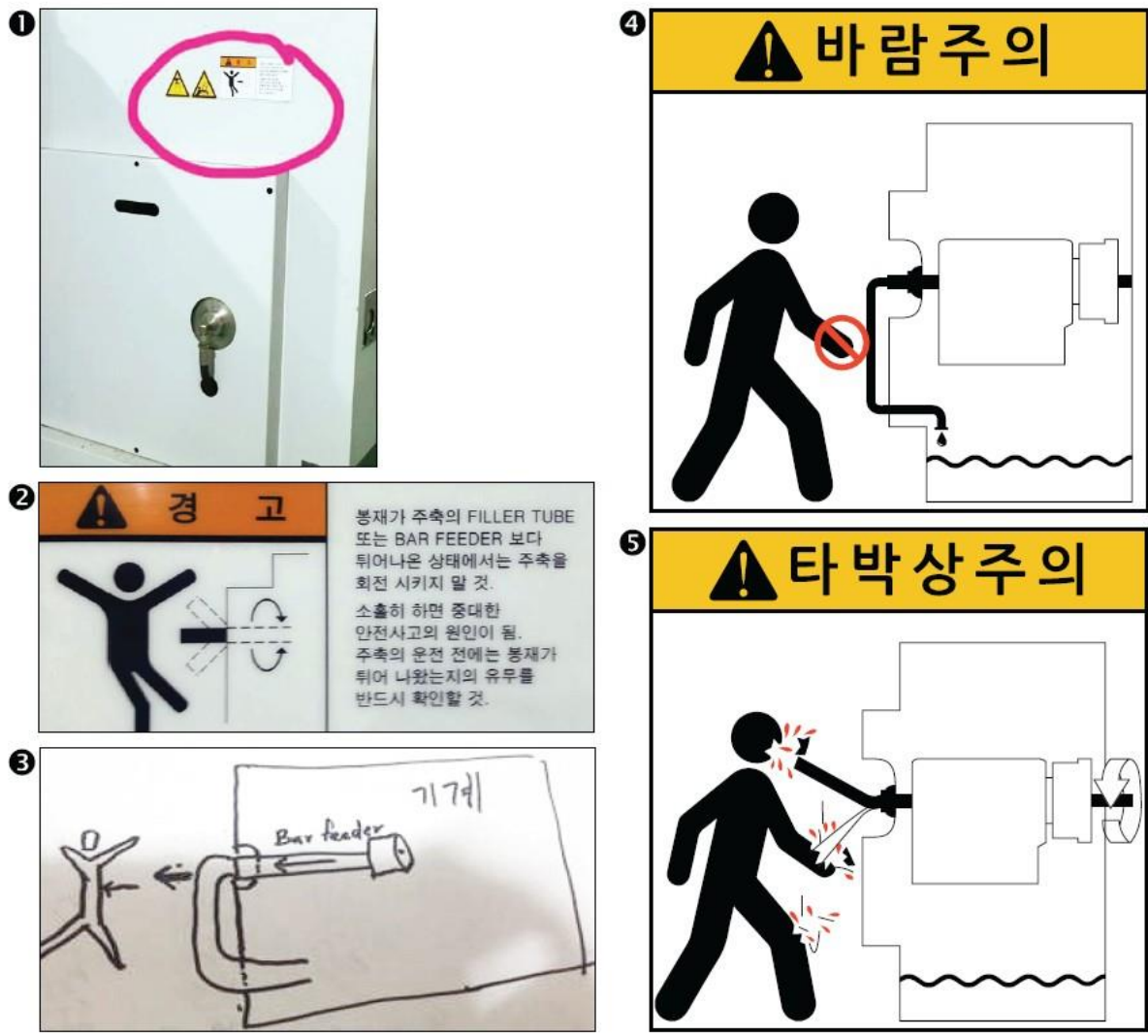
Figure 2. CNC machine safety sign, redesigned in collaboration with a participant: (1) a participant (SP 05) posted pictures. (2) current safety sign and captions. (3) the participant sketched what he wants to see to prevent accidents caused by strong wind. (4) a final sign warning against touching rubber tube and letting out strong wind. (5) a final sign warning about accidents caused by rotating bar end.
