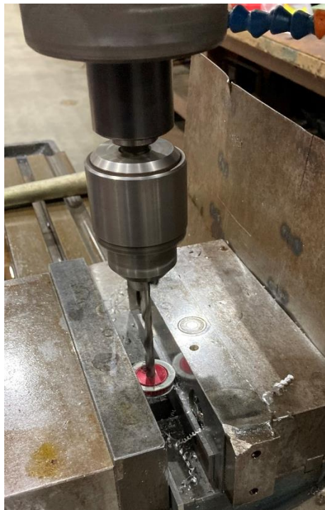
Figure 45: Increasing Center Hole for Shaft, Weapon Pulley, Fabrication
