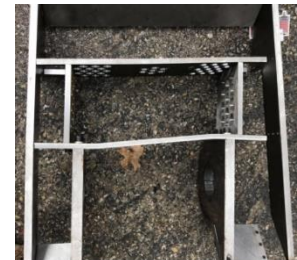
Figure 10: Frame Drop Test Damage
