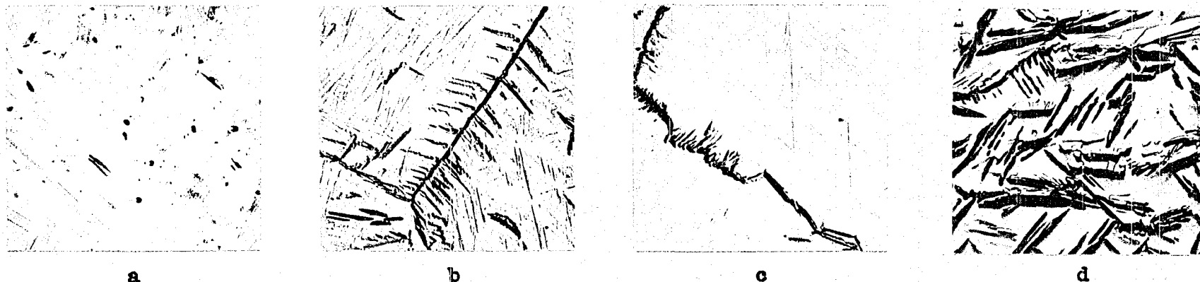
Figure 28. CE 14 Transformed at 825°C. for the Times Indicated.
