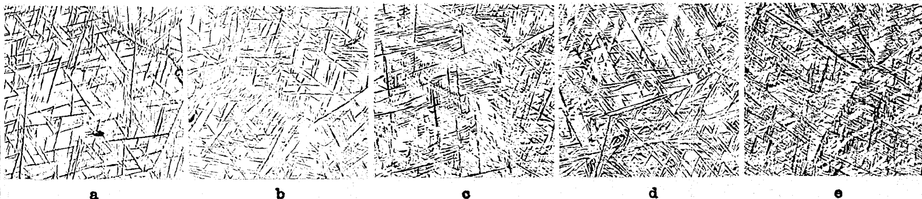
Figure 30. GE 14 Transformed at 720°C. for the Times Indicated. X 500
