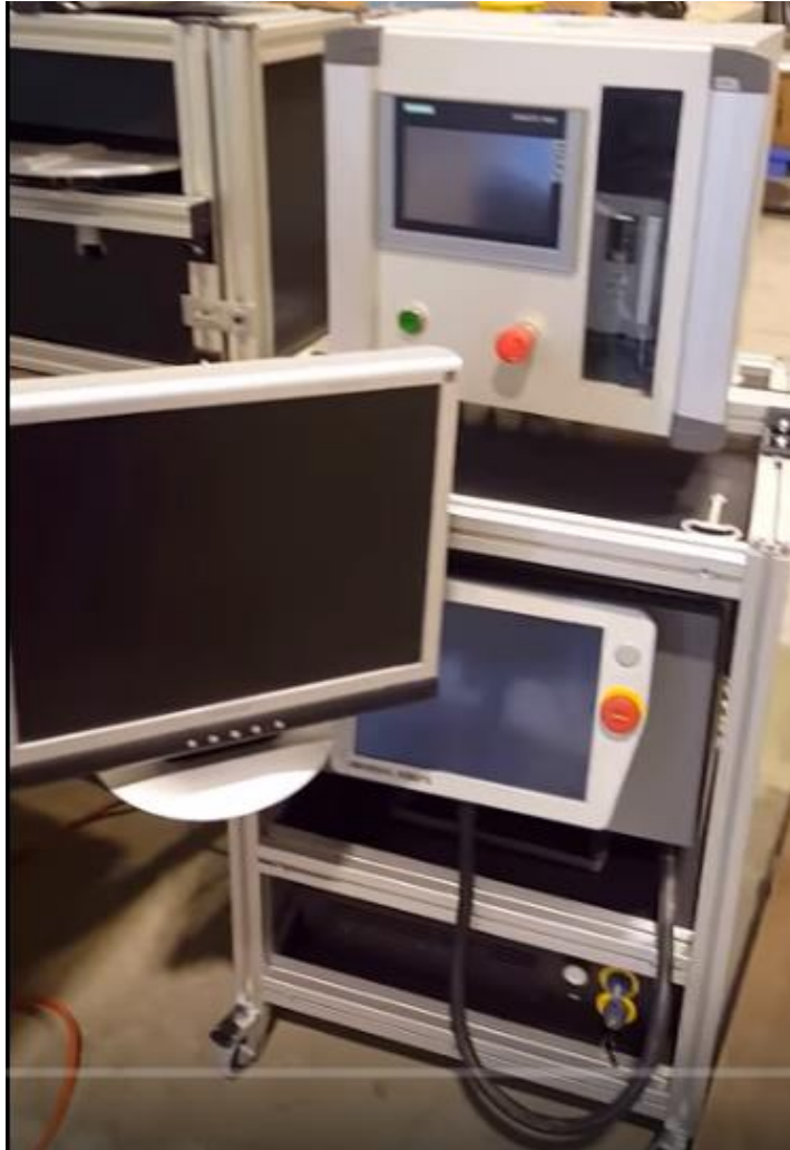
| Figure 17: Electrical Control Stand Assembled
