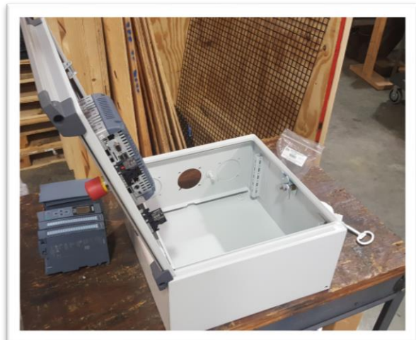
| Figure 9: Pre-Assembled Electrical Enclosure
