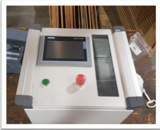
Figure 10: Electrical Enclosure Faceplate
