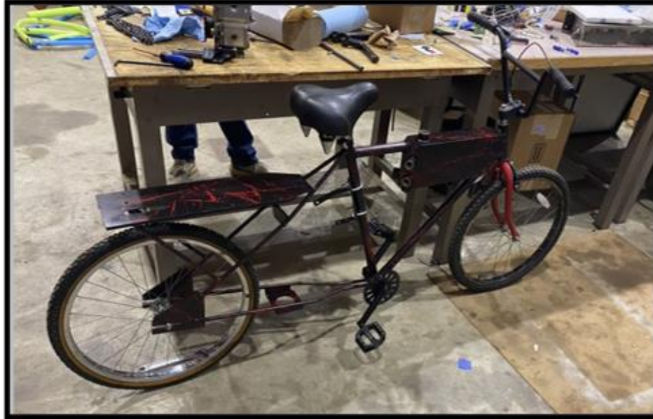
Figure 15: Final Fabricated Frame Design
