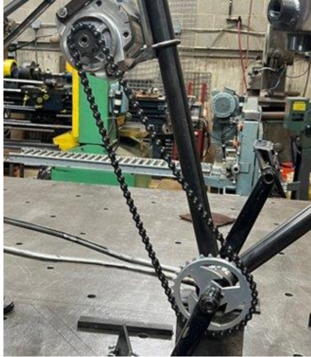
Figure 16: Peddle Sprocket going up to Tandem Sprocket
